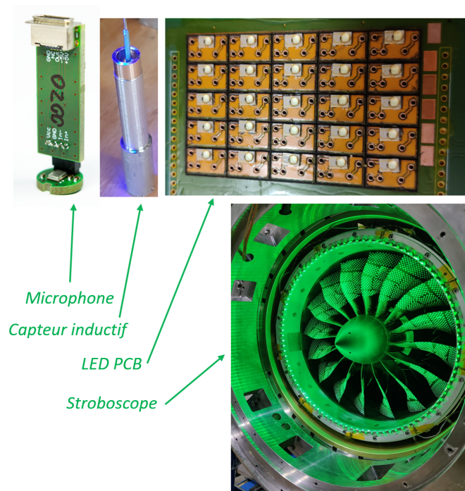
Figure 1. Instrumentation developed for the characterisation of NSV (Non-Synchronous-Vibration): Microphone, capacitive sensor for tip timing and tip gap measurement, LED PCB for stroboscope application.
