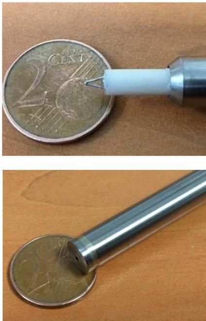
Figure 4: Temperature probe edge (top) and gas sampling probe end (bottom)
