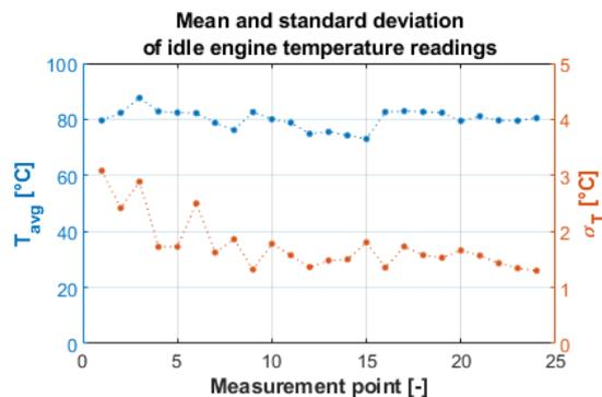
**FIGURE 8: MEAN AND STANDARD DEVIATION OF THE 24 CURATED IDLE ENGINE TEMPERATURE READINGS**
