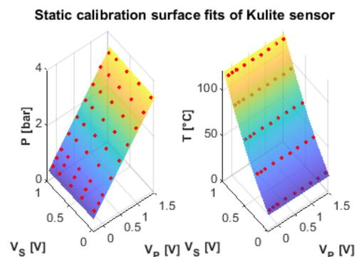
**FIGURE 3:** STATIC CALIBRATION OF KULITE SENSOR – PRESSURE (LEFT) AND TEMPERATURE (RIGHT) SURFACE FITS
