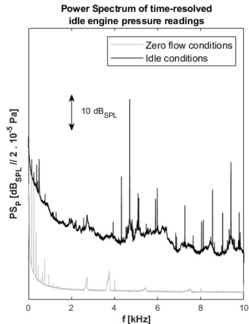
**FIGURE 9: POWER SPECTRUM OF IDLE ENGINE PRESSURE READINGS**
