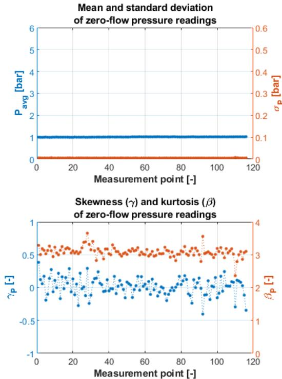
FIGURE 5: STATISTICAL MOMENTS OF ALL 116 ZERO-FLOW PRESSURE READINGS
