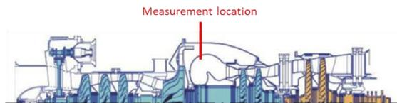
**FIGURE 2:** SAFRAN TECH BEARCAT TEST RIG [10] – SAFRAN HELICOPTER ENGINES MAKILA TURBOSHAFT GAS TURBINE
