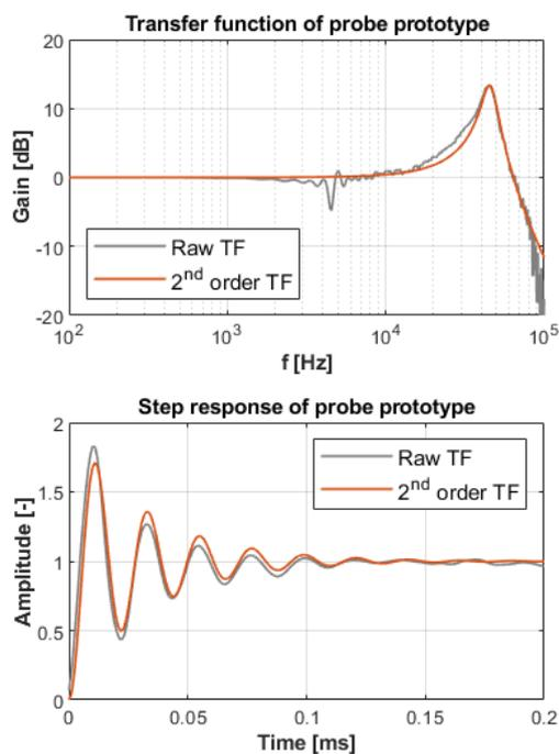
**FIGURE 4: DYNAMIC CALIBRATION OF PROBE PROTOTYPE**
