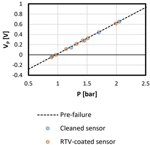
**FIGURE 10: SENSOR SENSITIVITY AT AMBIENT TEMPERATURE (T = 20°C)**
