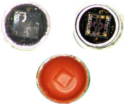
**FIGURE 11: SOOT-CONTAMINATED SENSOR (TOP LEFT) – CLEANED SENSOR (TOP RIGHT) – RTV-COATED SENSOR (BOTTOM)**
