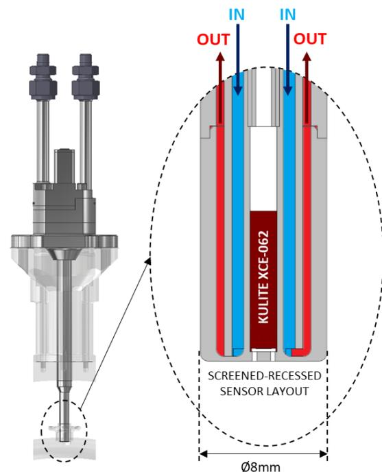
**FIGURE 1: PROBE DESIGN – COOLING LAYOUT AND SCREENED-RECESSED SENSOR LAYOUT**
