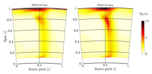
Figure 1. Turbulence at the exit of first stator with FRAP-4S 3mm (left) and 4mm tip diameter (right).
