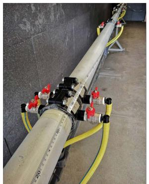
Figure 1. Experimental setup for pipe leakage detection and localization
