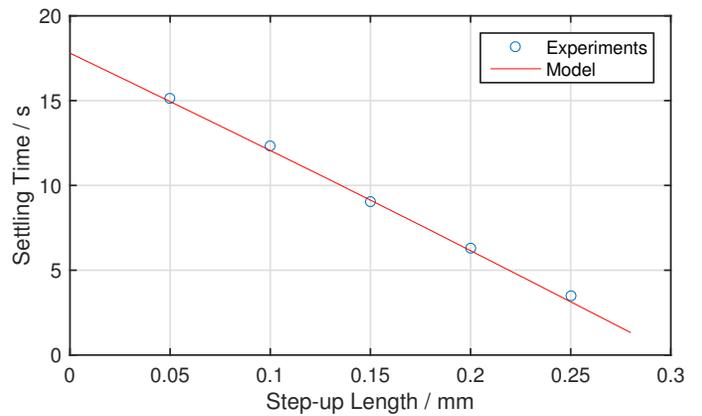
**FIGURE 12:** Measured and predicted settling time against step-up length.  $hd = 0.185$  mm,  $sd = 0.680$  mm,  $td = 1.00$  mm,  $tl = 3500$  mm
