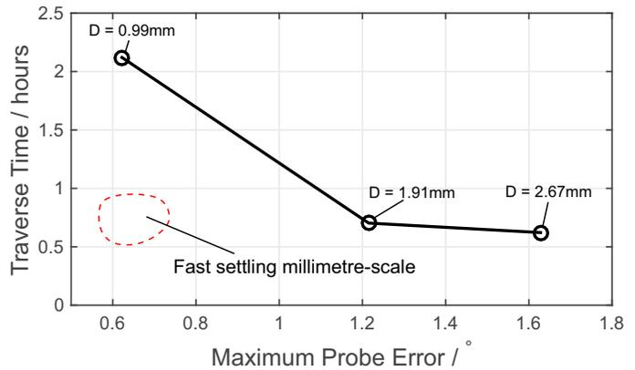
FIGURE 7: The trade between total traverse time and probe error
