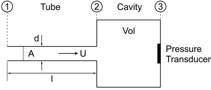
FIGURE 8: Tube connected to pressure transducer via a cavity
