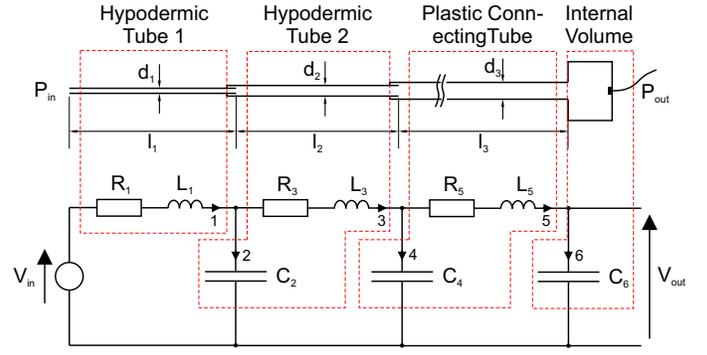
FIGURE 9: Probe with step-ups and analogous electric circuit
