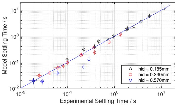
**FIGURE 11:** Comparison of measured and predicted settling times
