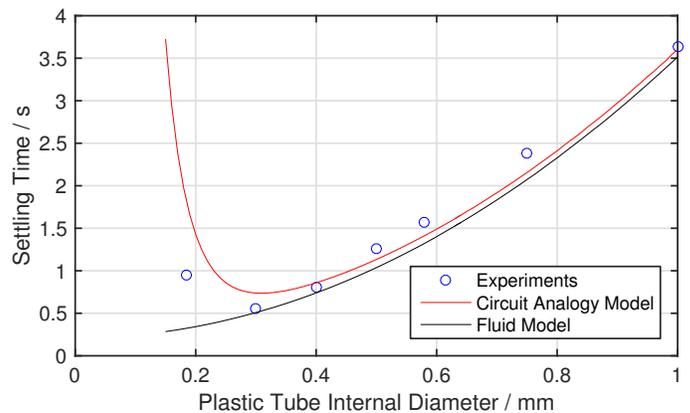
**FIGURE 13:** Measured and predicted settling time against plastic tube internal diameter.  $hd=0.185$  mm,  $hl=200$  mm,  $tl=1000$  mm
