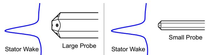
b) Small five-hole probes have a long settling time
