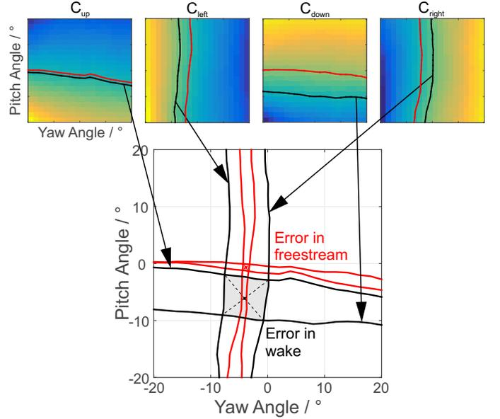
**FIGURE 4:** Top: Formulation of side coefficients and possible angle functions. Bottom: Error estimate taken from quadrilateral diagonal length. Both from 2.67 mm probe
