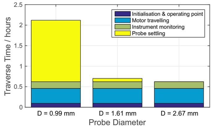
FIGURE 6: Breakdown of traverse times with different size probes
