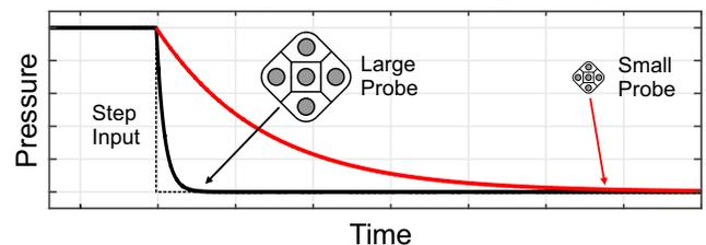
FIGURE 1: Trade between accuracy and traverse time in five-hole probe design
