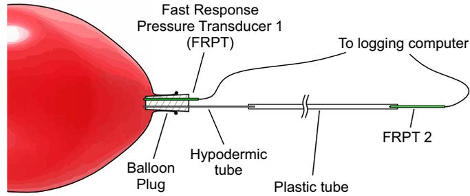
**FIGURE 10:** Experimental setup for measuring settling time of pneumatic probes
