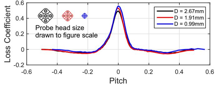
**FIGURE 3:** Measured midspan stator wake loss coefficient
