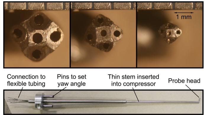
**FIGURE 2:** Top: Microscope view of probe head geometry. Bottom: Overview of probe design
