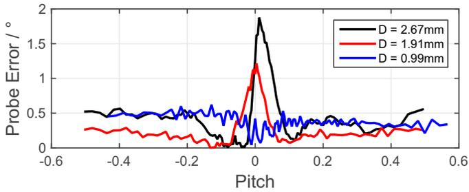
FIGURE 5: Calculated probe error in stator midspan wake
