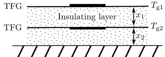
**Figure 10:** Self-heating gauges.
