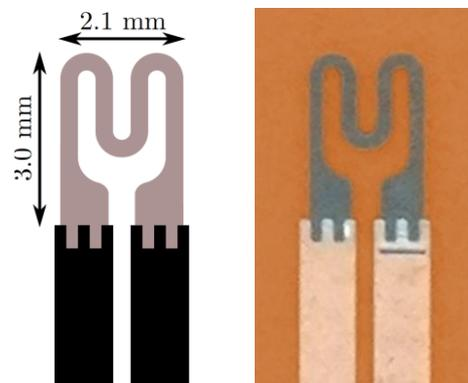
Figure 1: Gauge dimensions and photograph.
