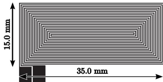
**Figure 4:** Example of a heater design.
