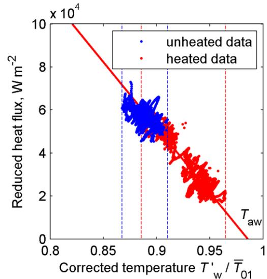
**Figure 8:** Regression data for one double-sided gauge with an underside heater compared to unheated results.
