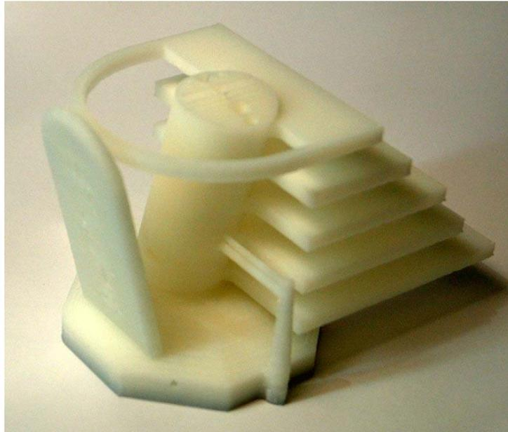
**Figure 2. Dimension SST test part.**
