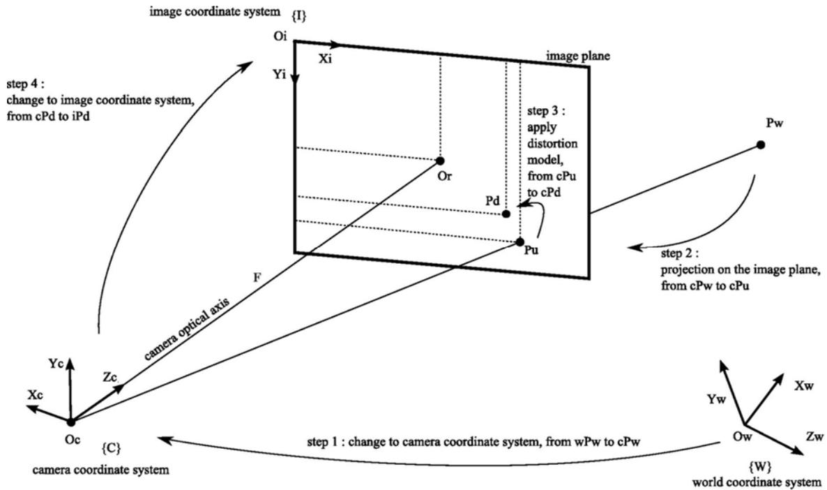
Fig. 7: Camera calibration principle.
