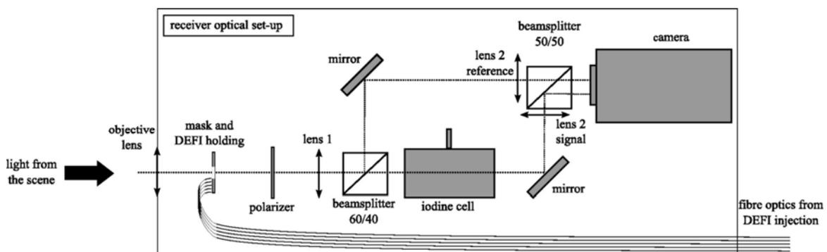
Fig. 3: Optical setup of the reception part of the DGV system.
