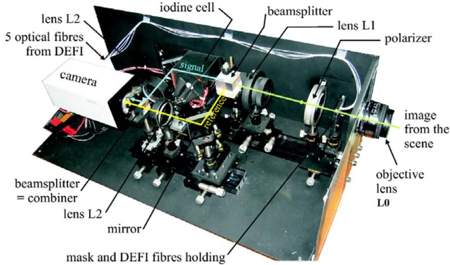
**Fig. 6: Receiver setup.**
