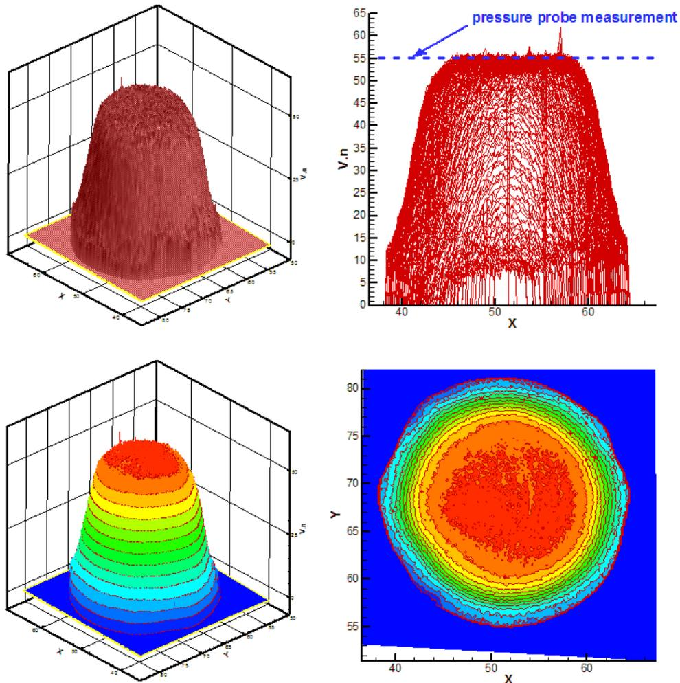
**Fig. 9: Axial velocity distribution in a round free jet –  $x/d = 1.0$ .**
