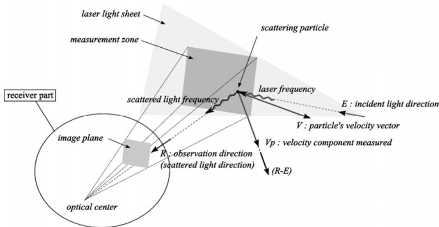
Fig. 1: DGV principle for measuring the component  $V_p$  on  $(R - E)$  of the particle's velocity vector  $V$ .
