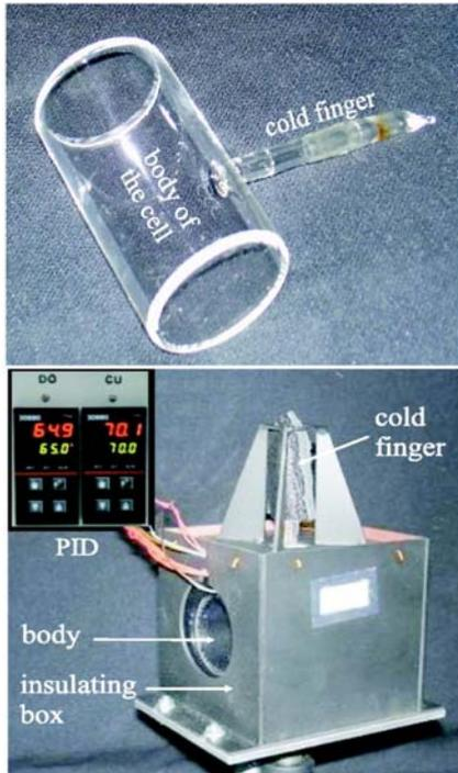
Fig. 4: Iodine cell (top) and iodine cell in its insulated box with its PID controller (bottom).
