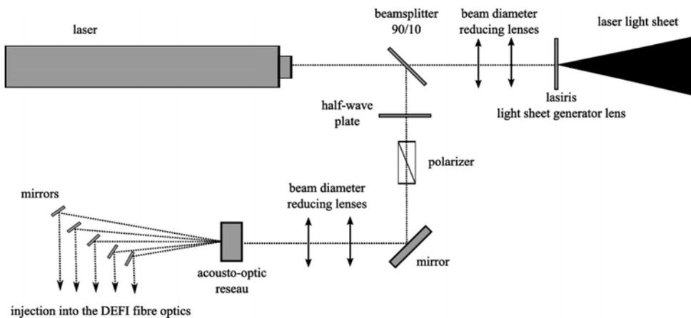
Fig. 2: Optical setup of the emission part of the DGV system.
