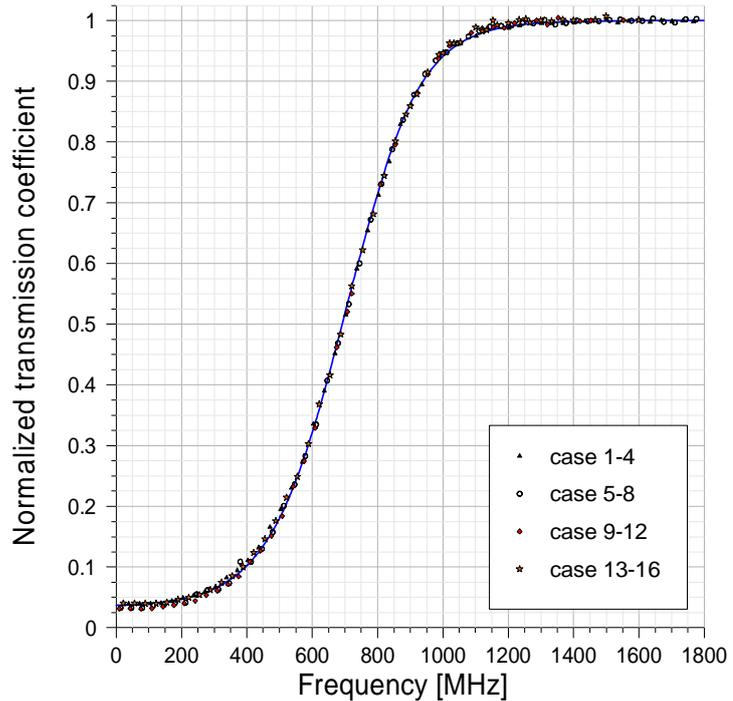
Fig. 5: Normalized transmission coefficient obtained in the right flank of iodine cell absorption line.
