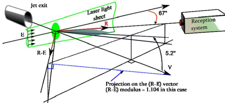
*The zone of the DGV image that concerns the seeded area is defined with  $172 \times 182$  pixels, corresponding to a square in the world frame of  $30 \times 30$  mm<sup>2</sup>.*
