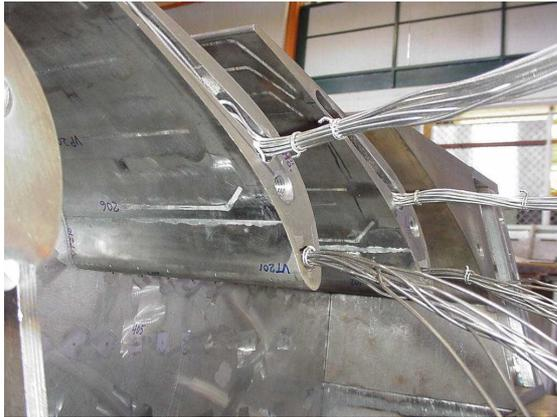
**Figure 7: Instrumented airfoils**
