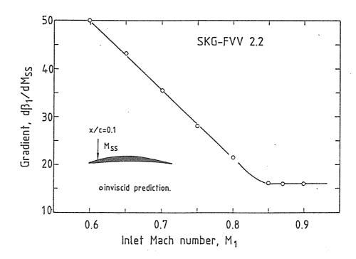
Fig.4 Gradient dB<sub>1</sub>/dM versus inlet Mach number of a Controlled Diffusion Airfoil
