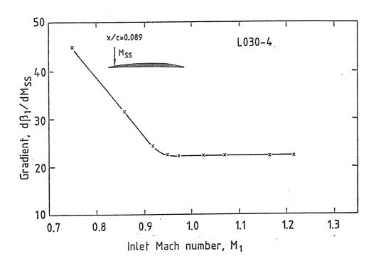
Fig.12 Gradient  $d\beta_1/dM$  versus inlet Mach number of an MCA blade section
