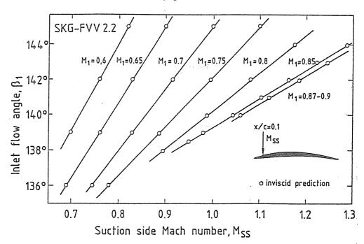
Fig.3 Inlet flow angle versus surface Mach number of a Controlled Diffusion Airfoil
