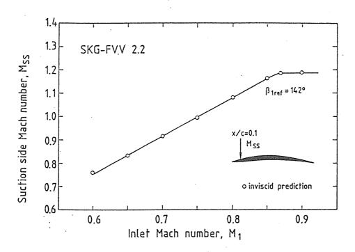
Fig.7 Suction side Mach number versus inlet Mach number of a Controlled Diffusion Airfoil
