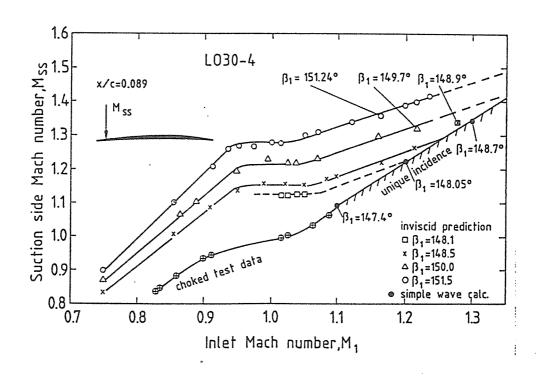
Fig.11 Suction side Mach number versus inlet Mach number of an MCA blade section
