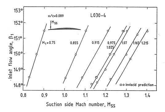
Fig.10 Inlet flow angle versus surface Mach number of an MCA blade section
