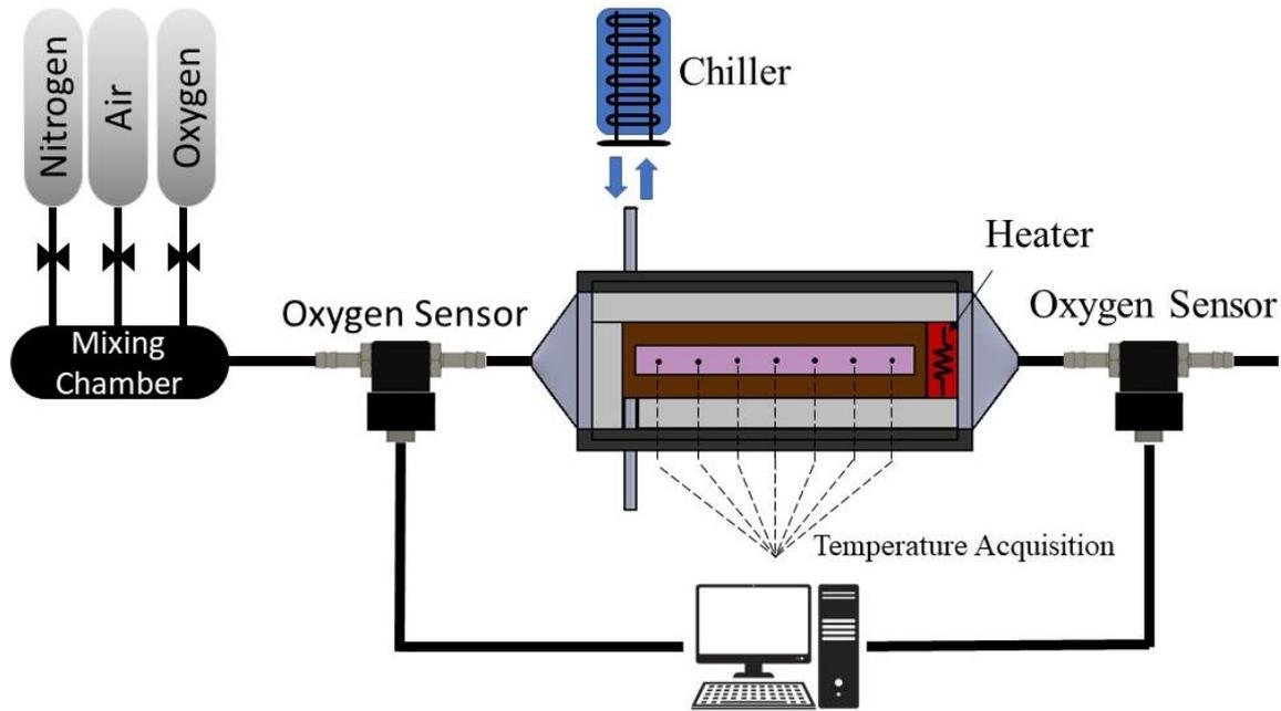
Figure 3. PSP calibration system schematic
