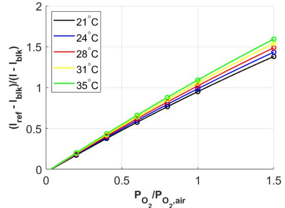
Figure 8. UniFIB one-dimensional calibration map for five different temperatures.
