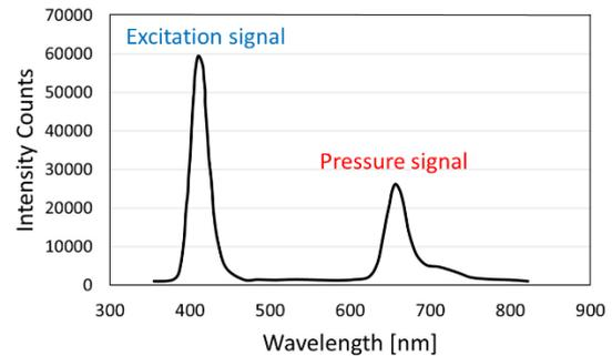
Figure 1. Spectral response of the ISSI UniFiB PSP signal.
