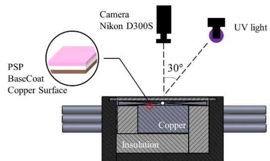
Figure 5. PSP calibration system front view schematic
