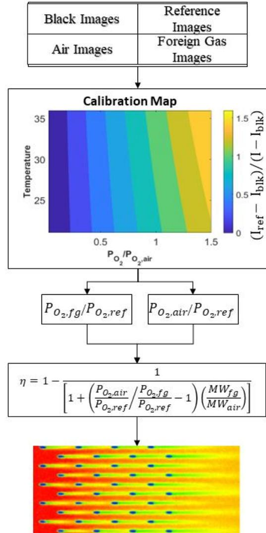
**Figure 6. Flowchart for PSP experimental procedure**
