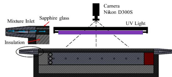
Figure 4. PSP calibration system side view schematic
