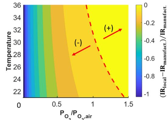
Figure 9. Comparison of the calibration map with the manufacturer's specifications.
