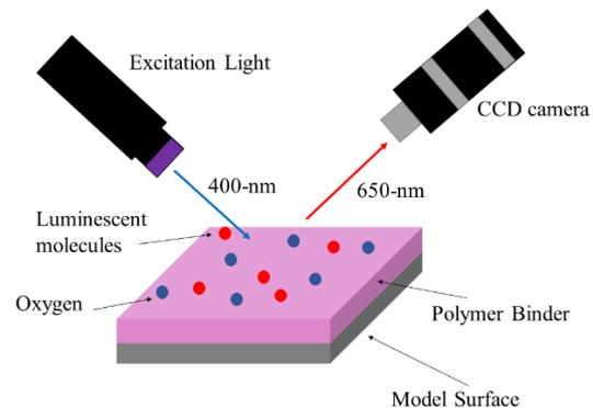
Figure 2. PSP system schematic
