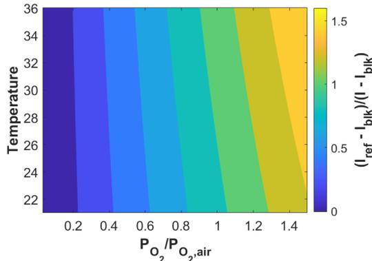
Figure 7. UniFIB two-dimensional calibration map
