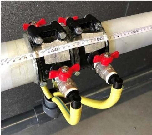
Fig. 3. Artificial leakages by means of valves and plastic tube that used to avoid any flooding inside the container
