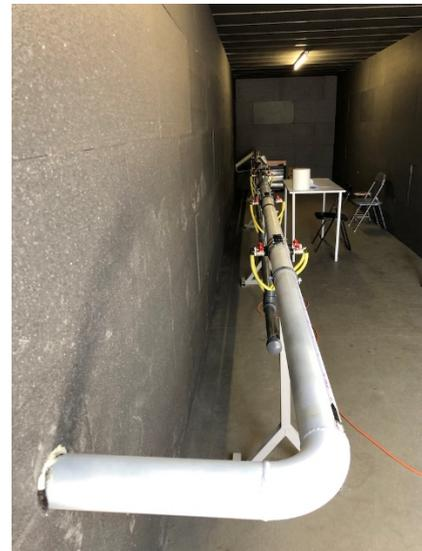
Fig. 2. Pipeline section inside the anechoic chamber
