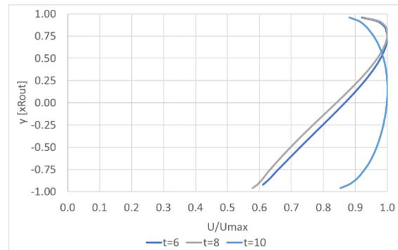
Figure 11: Effect of thickness on the flow profile 10D downstream the control valve
