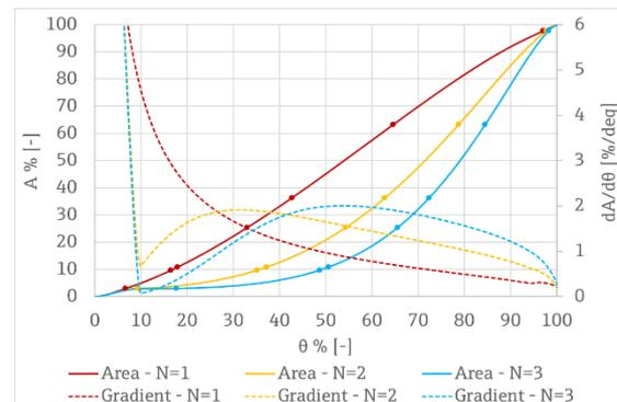
Figure 9: Effect of polynomial's order  $N$  on the control valve's characteristics
