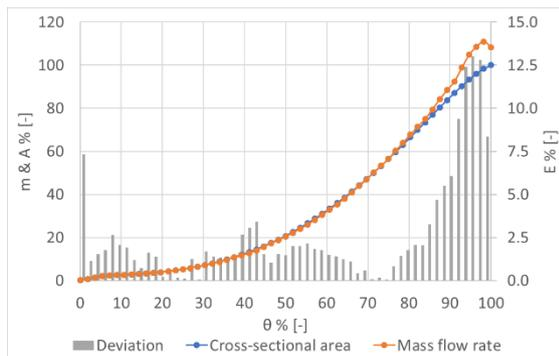
Figure 14: Percentagewise comparison of cross-sectional area and mass flow of the control valve
