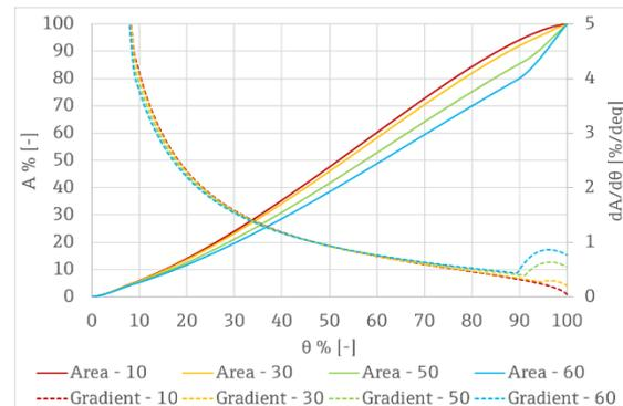
Figure 8: Effect of radius  $\Delta\theta_c$  on the control valve's characteristics
