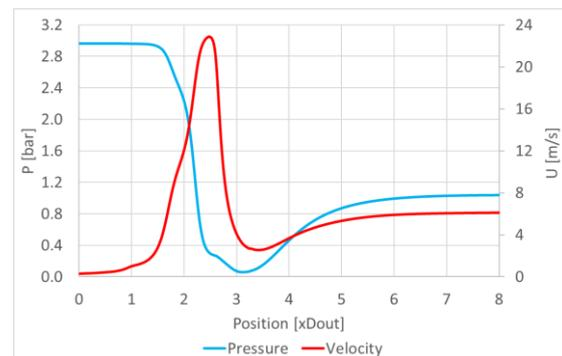
Figure 12: Pressure and velocity variation across the control valve
