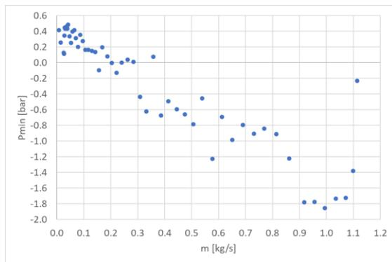
Figure 13: Minimum pressure for various flow rates
