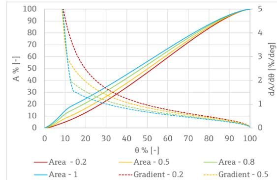
Figure 7: Effect of radius  $R_1$  on the control valve's characteristics
