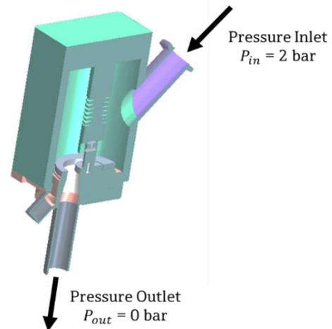
Figure 1: Control valve model
