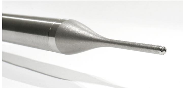
**Figure 3. Fast-response five-hole probe equipped with piezo-resistive sensors**
