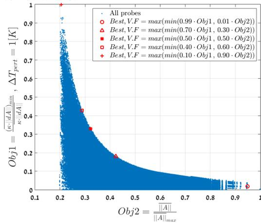
Figure 4 – Map of the two objectives for all 4-wire probes combinations
