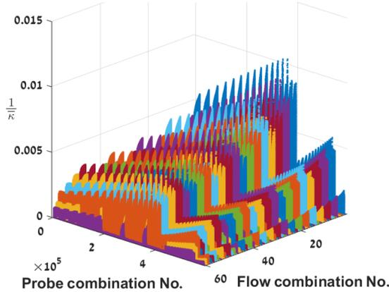
Figure 1 – Inverse condition number of all 4 wire probe combinations for broad range of mean flow properties
