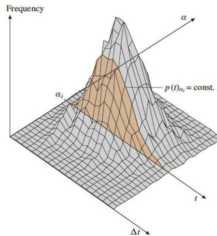
**Figure 6.** Two-dimensional histogram at different angles of the measuring plane (Tropea et al. 2007)
