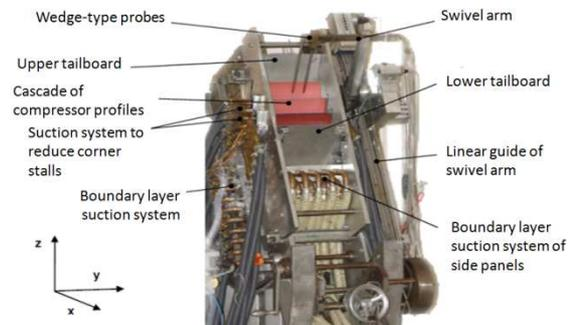
**Figure 7.** Cascade wind tunnel at the TFD
