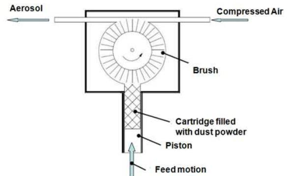
**Figure 9.** Functional principle of particle disperser
