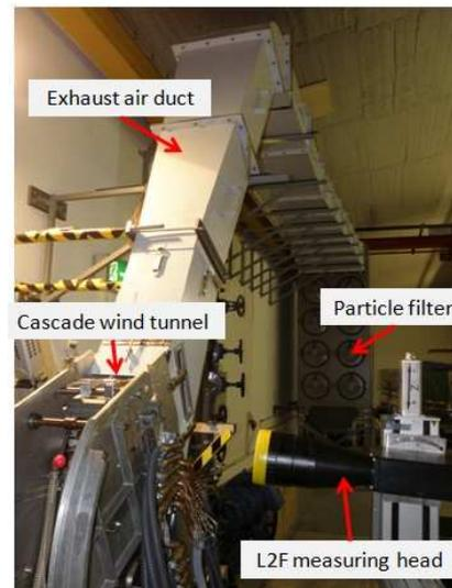
Figure 1. Cascade wind tunnel at the TFD
