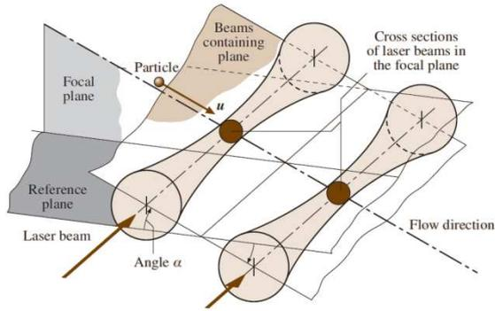
**Figure 4.** Measuring plane of L2F-method (Tropea et al. 2007)
