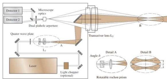
**Figure 2.** Layout of typical L2F-velocimeter (Tropea et al. 2007)
