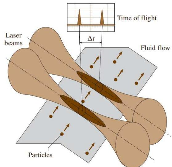
**Figure 3.** Time-of-flight velocimeter probe volume (Tropea et al. 2007)
