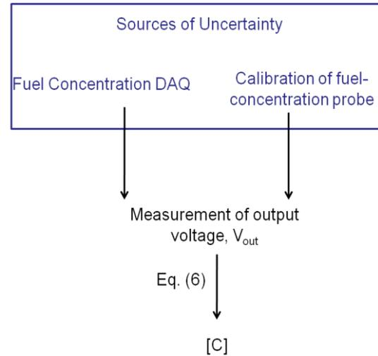
Fig. 7 Uncertainty propagation during fuel concentration measurements.
