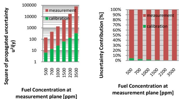
Fig. 11 Square of propagated uncertainties  $u^2_i(y)$  on logarithmic axis (left) for 6 different fuel concentrations [ppm] and uncertainty contribution of calibration and measurement (right).
