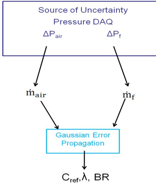
Fig. 3 Uncertainty propagation during pressure measurements
