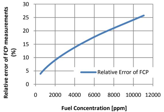
Fig. 10 Percentage of relative error ( $e_r$ ) for different values of fuel concentration
