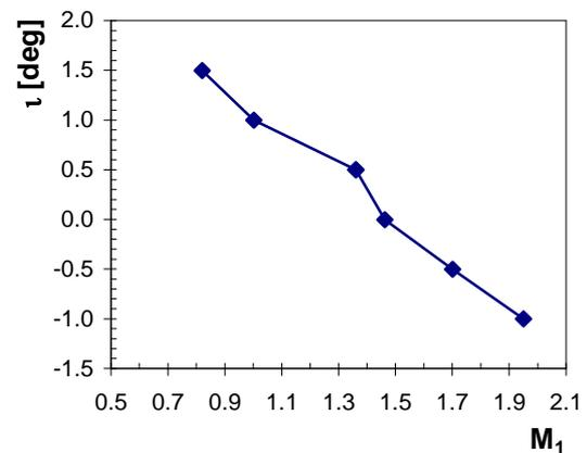
**Fig. 5:** Dependence of inlet angle on inlet Mach number for typical tip section of a long rotor blade (Fig. 4). Result of CFD.
