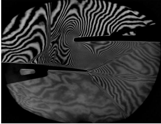
**Fig. 9:** Interferogram taken at  $M_{2is} = 1.674$  and  $M_I = 1.066$ . Upper wall suction off.
