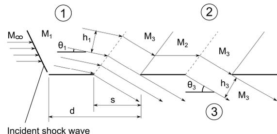
**Fig. 6:** Schematic of flow past perforated wall with incident shock wave [11].
