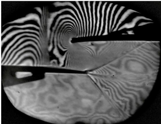
**Fig. 10:** Interferogram taken at  $M_{2is} = 1.689$  and  $M = 1.077$ . Upper wall suction on.
