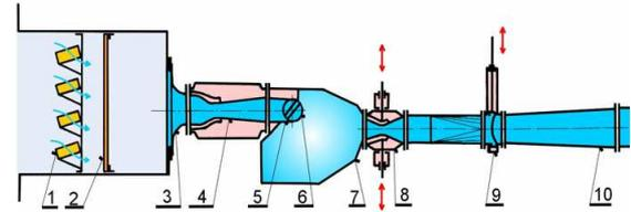
**Fig. 7:** Scheme of the suction type high-speed wind tunnel. 1 silicagel dryer, 2 filters, 3 entrance nozzle, 4 inlet nozzle, 5 transient insert, 6 rotatable test section, 7 settling chamber, 8 control nozzle, 9 quick-acting valve, 10 diffuser, 11 main duct
