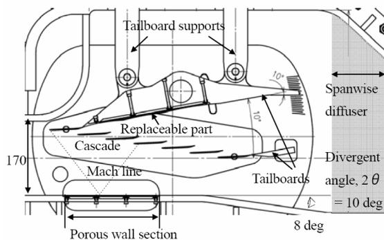
**Fig. 2:** Test section used for turbine blade tip aerodynamic tests by Shibata et al. [10]
