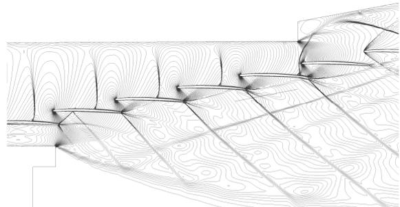
**Fig. 13:** Numerical simulation of the flow past turbine blade tip cascade model in the wind tunnel with test section consisting of no devices improving supersonic inlet and outlet flow. Reprinted from [15]
