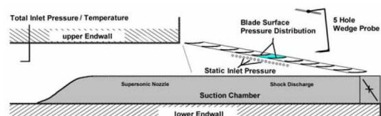
**Fig. 1:** Test section used for turbine blade tip aerodynamic tests by Parvizinia et al. [8]
