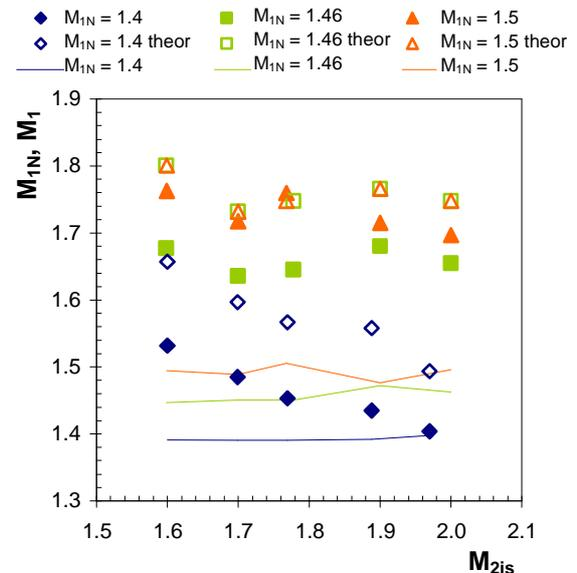
Fig. 16: Dependencies of nozzle inlet Mach numbers (measured and theoretical) and cascade inlet Mach numbers on isentropic exit Mach number
