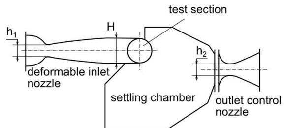
**Fig. 14:** Scheme presenting the wind tunnel as a channel with two aerodynamic throats.
