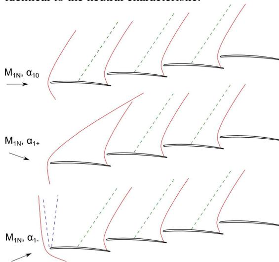
**Fig. 4:** Self adjustment of unique incidence conditions at inlet when incidence angle of the flow coming from the nozzle is equal, higher or lower than the unique value.
