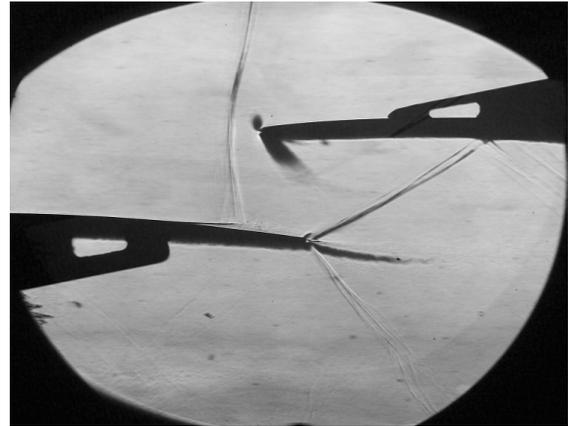
**Fig. 12:** Schlieren picture taken at  $M_{2is} = 1.798$  and  $M_I = 1.257$ . Perforated tailboard applied and set to an angle  $\alpha_{pt} = 15.75^\circ$
