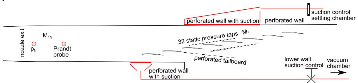
**Fig. 8:** Test section for measurements on supersonic turbine blade tip cascades
