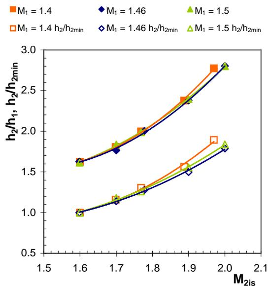
**Fig. 17:** Wind tunnel characteristics - dependencies of the wind tunnel setting upon isentropic exit Mach numbers  $M_{2is}$  for several cascade inlet Mach numbers  $M_1$
