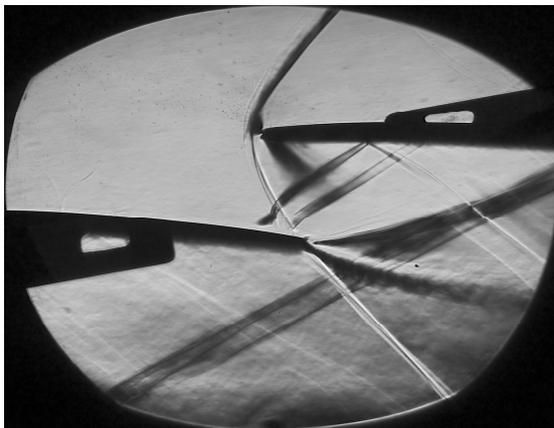
**Fig. 11:** Schlieren picture taken at  $M_{2is} = 1.838$  and  $M_I = 1.29$  showing shock wave reflected from the free jet boundary when no perforated tailboard is applied.
