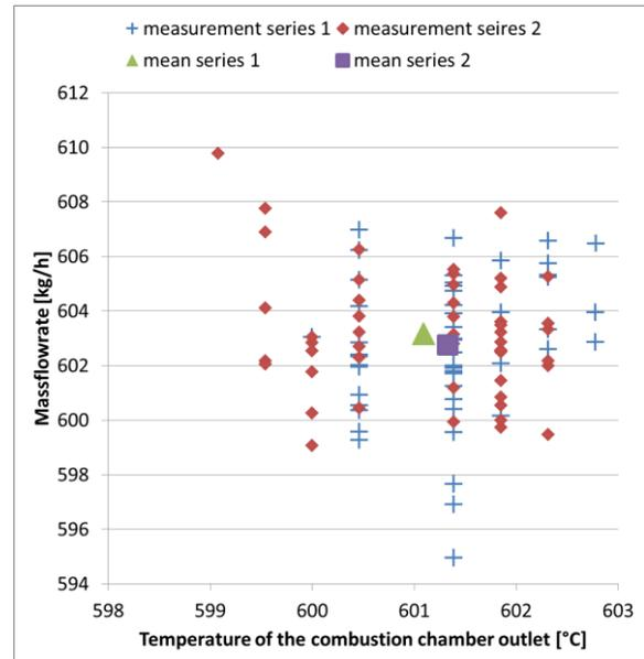
Figure 5: Reproducibility and accuracy of temperature and mass flow
