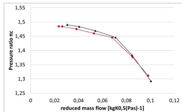
Figure 6: Reproducibility of compressor map - pressure ratio
