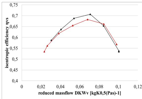
Figure 7: Reproducibility of compressor map - efficiency
