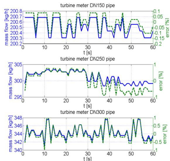
**Figure 2: accuracy of the turbine meters in the compressor suction pipe**
