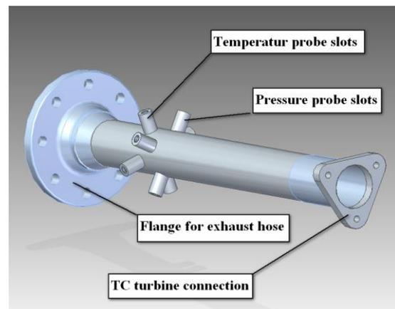
Figure 4: Measurement pipe at TC turbine outlet
