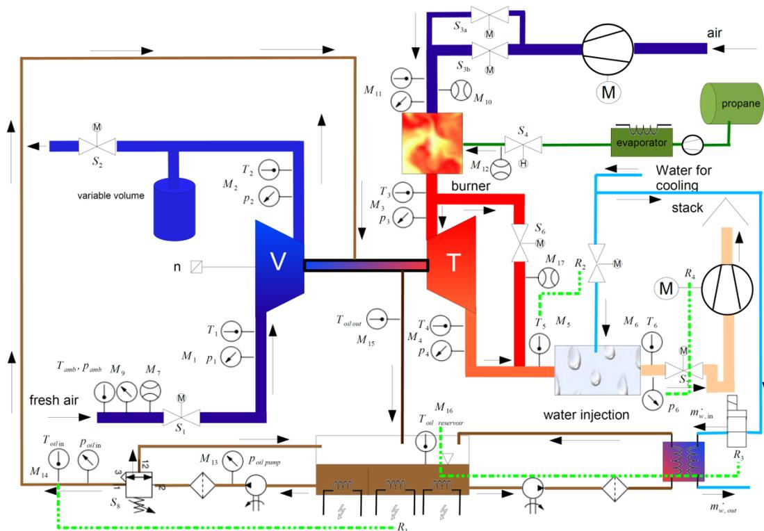
Figure 1: Schematic diagram of the ITSM turbocharger test facility
