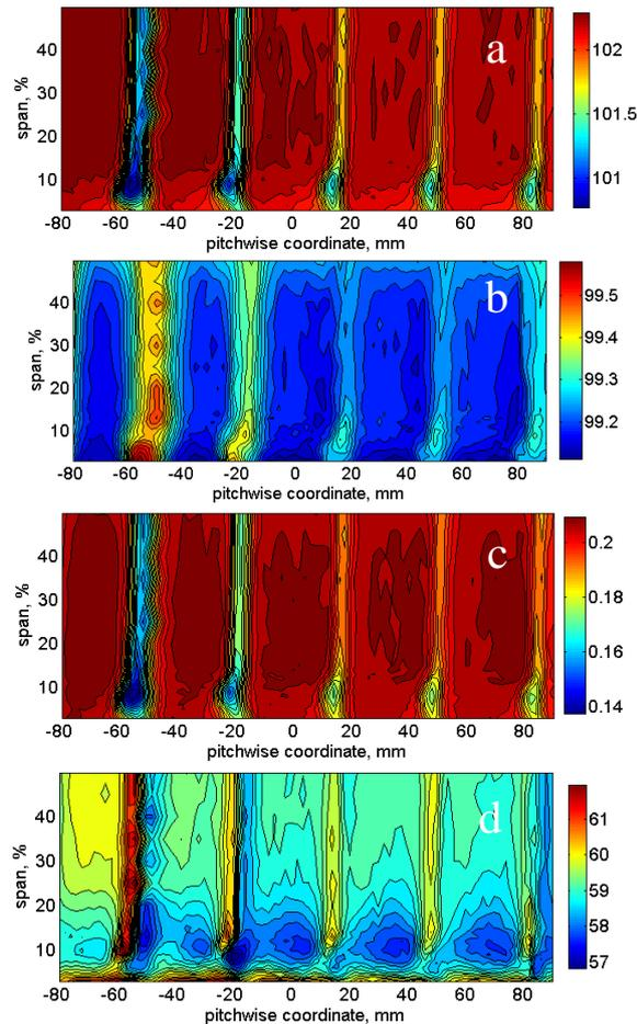
**Figure 7: Downstream distributions of (a) total pressure [kPa]; (b) static pressure [kPa]; (c) Mach number; (d) flow angle [deg]**
