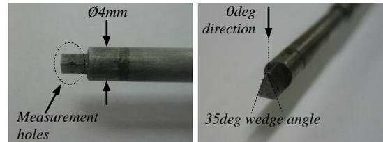
**Figure 3: Aerodynamic 3-hole wedge probe**
