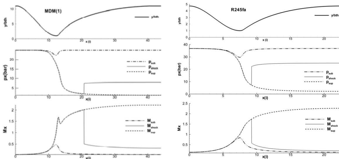
**Figure 9: Pressures and Mach trends along the axial coordinate of the nozzle for three different LPV pressure values. Left MDM(1), Right R245fa.**
