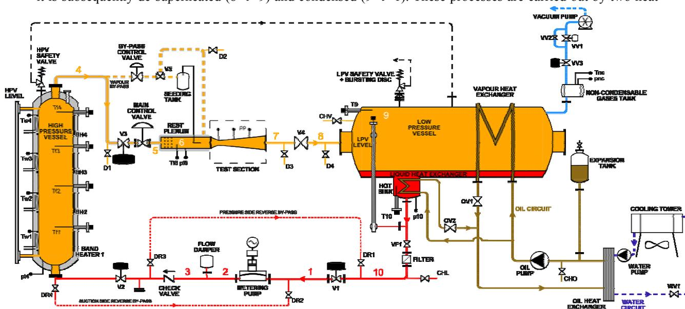
Figure 4: Final layout of the Test Rig for Organic Vapours
