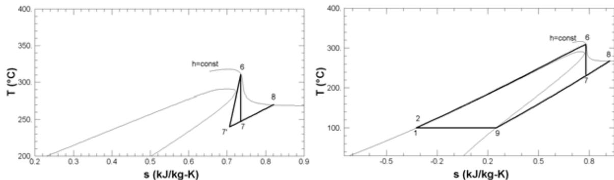
**Figure 2: Options for Test Rig continuous cycle. Left: gas cycle. Right: phase transition cycle**
