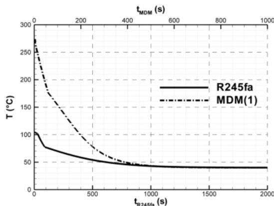
**Fig. 10: Temperature trends of MDM(1) and R245fa during the condensation process**
