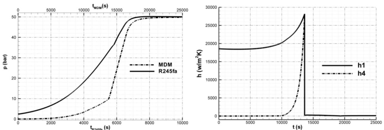
**Figure 6: Left: pressure trends of MDM(1) and R245fa within HPV. Right: heat transfer convective coefficients for MDM(1) in lower ( $h_1$ ) and upper ( $h_4$ ) HPV zones**
