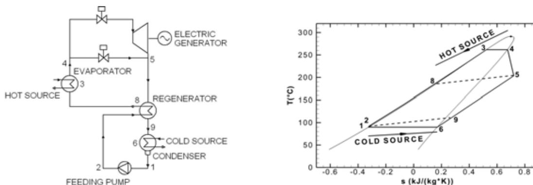
Figure 1: Left: Typical regenerative Organic Rankine Cycle power plant.
