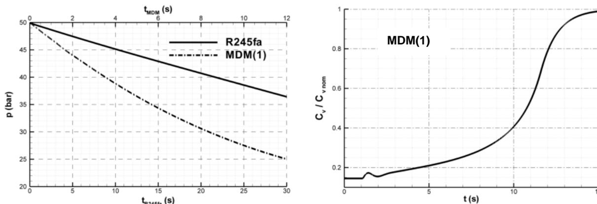
Figure 7: Left: HPV pressure trends for MDM(1) and R245fa tests.
