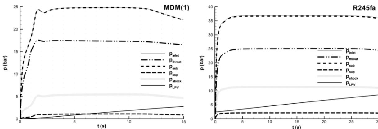
Figure 8: Pressure threshold values for MDM(1) (left) and R245fa (right) tests
