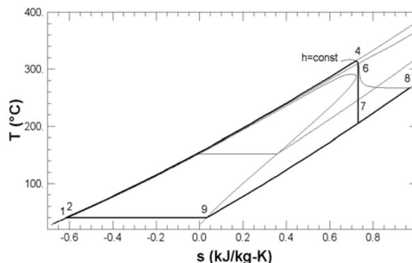
Figure 3: Test Rig thermodynamic cycle
