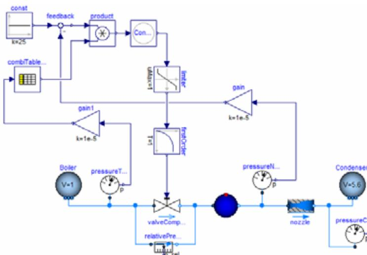
Figure 5 : Dymola model of the test including the control loop
