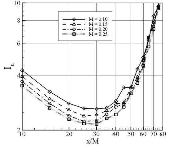
Figure 8: Evolution of streamwise turbulence intensity along the jet
