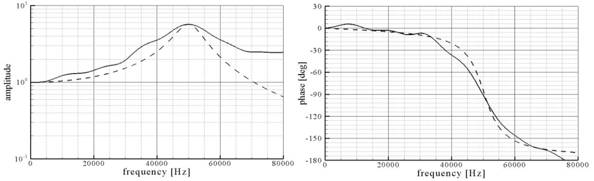
**Figure 2: Experimental transfer function of the total pressure probe evaluated in shock tube tests (solid line) and identification as second-order linear system (dashed line)**
