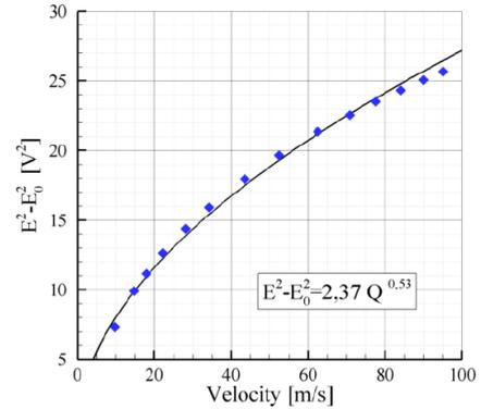
Figure 3: Hot wire calibration curve
