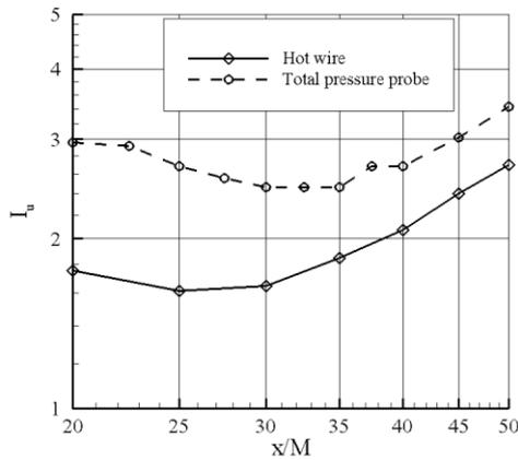
**Figure 9: streamwise turbulence intensity along the jet. Comparison between hot wires and pressure probe**
