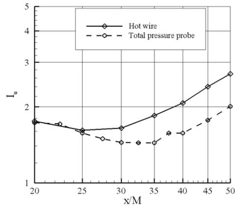
**Figure 10: streamwise turbulence intensity along the jet. Comparison between hot wires and pressure probe after recovery correction**
