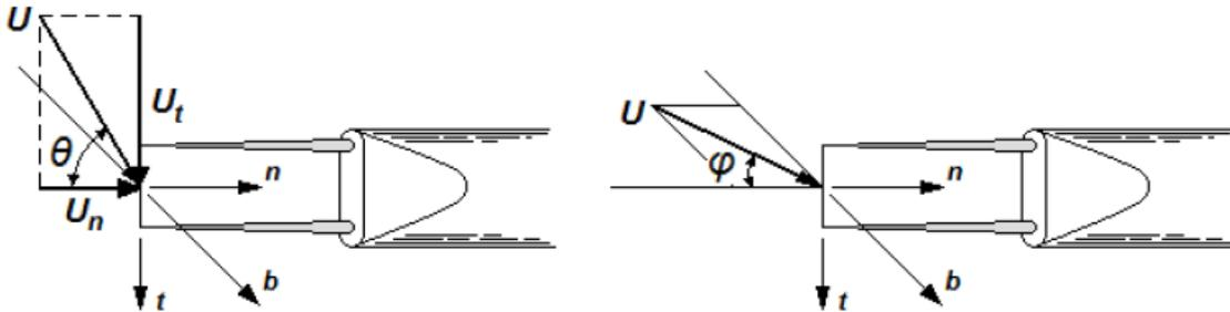
Figure 4: Intrinsic reference frame for normal hot wire probes
