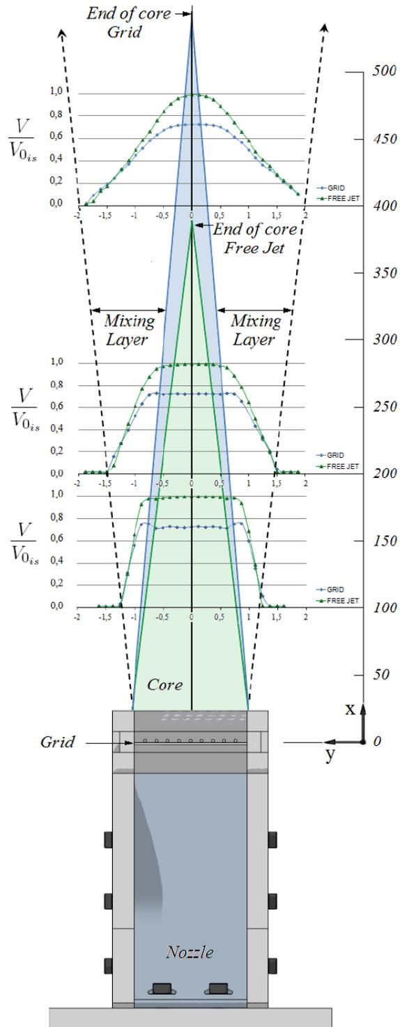
Figure 7: Jet development in streamwise direction
