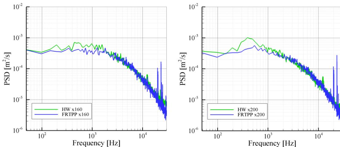
**Figure 11: Power Spectrum Density from hot wires and total pressure probe (recovery corrected data). Left,  $x/M = 20$ ; Right,  $x/M = 25$**
