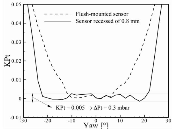
Figure 1: Aerodynamic behaviour of the FRTPP with flush mounted or recessed sensors
