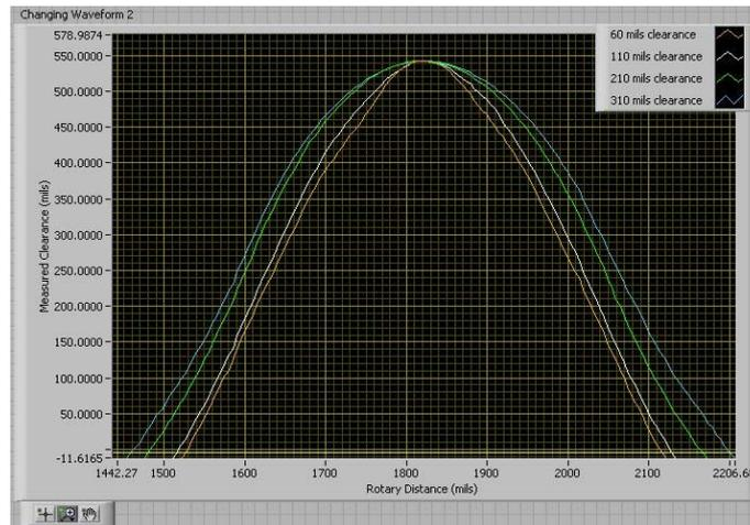
**Figure 4. Measurement of a simplified blade at several clearances showing the blurring effect of spatial filtering.**
