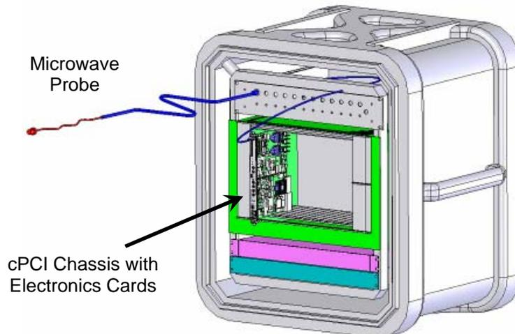
**Figure 1. Representation of microwave tip clearance system**
