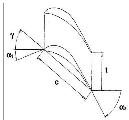
Fig.2: SE1050 linear blade cascade configuration (©VZLU)
