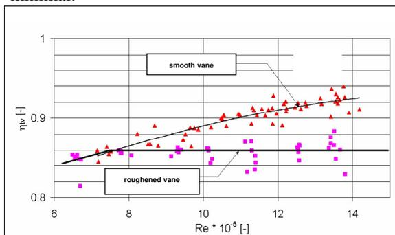
Fig.10: Sand-roughness impact on turbine stage efficiency (stator wheel roughened,  $Ra = 0.8, 9$ )
