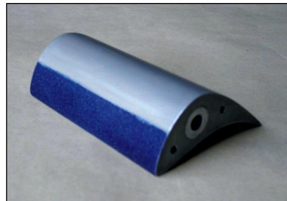
Fig.5: Sand-roughness applied to the VS33 vane
