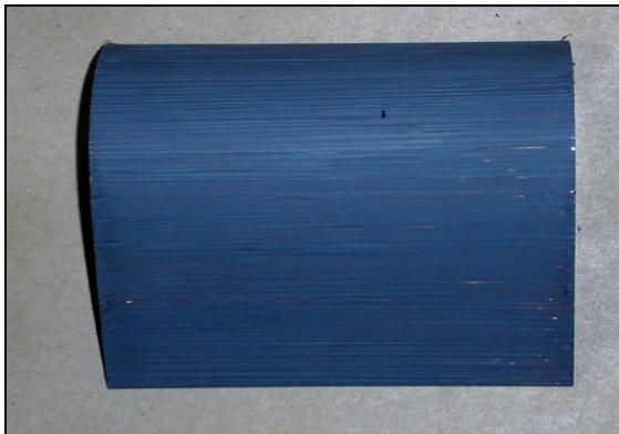
Fig.4: Oriented roughness applied to the VS33 vane
