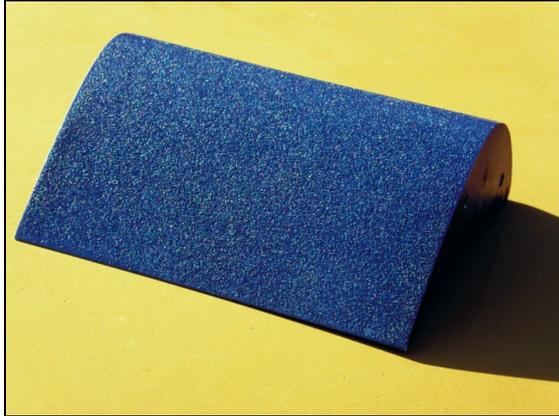
Fig.3: Sand-roughness applied to the VS33 vane ( $R_a = 30$ )
