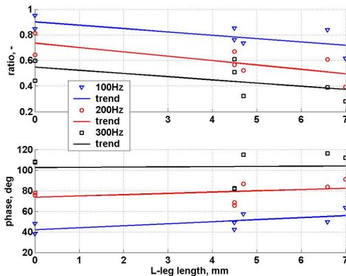
Figure 10. Effect of length of L-leg
