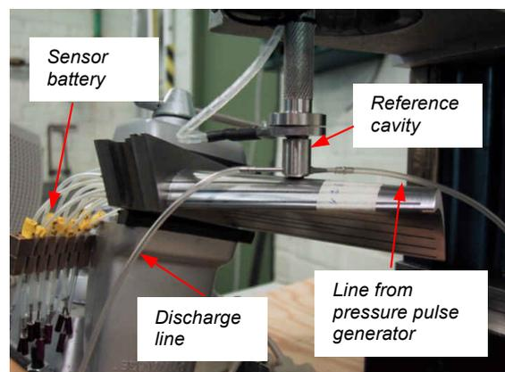
**Figure 7.** Calibration setup
