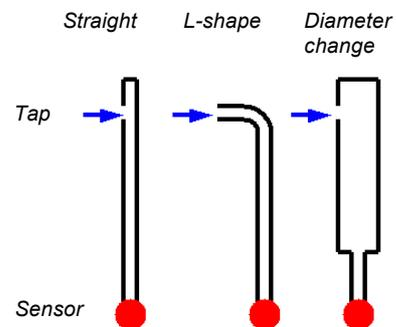
Figure 4. Shapes of connection tubes
