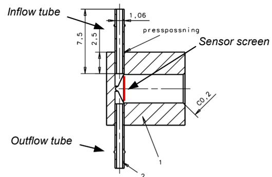
Figure 5. Section through sensor battery
