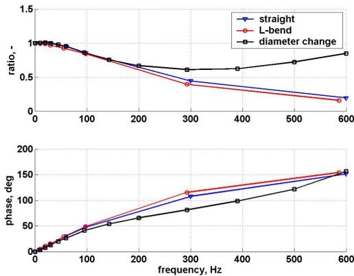
Figure 9. Effect of tube shape
