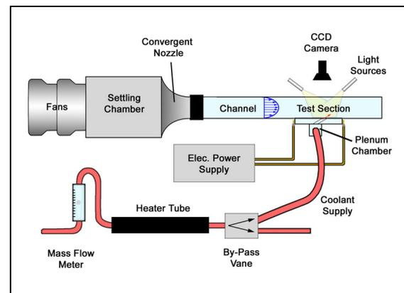
**Fig. 1: Schematic drawing of the test facility.**
