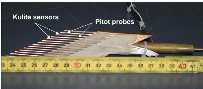
Fig. 3: Wake rake with *Kulite* sensors and conventional pitot probes
