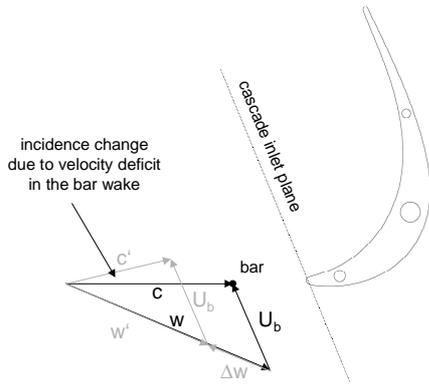
Fig. 10: Schematic velocity triangle in the cascade inlet plane with and without wakes
