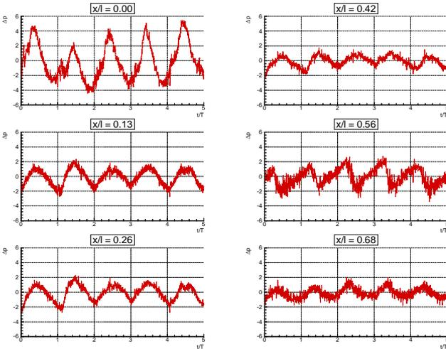
Fig. 11: Ensemble-averaged time traces of fluctuating pressure on the suction side for  $Ma_{2th} = 0.4$ ,  $Re_{2th} = 200,000$ ,  $t_b = 80$  mm,  $U_b = 10.7$  m/s, no grid
