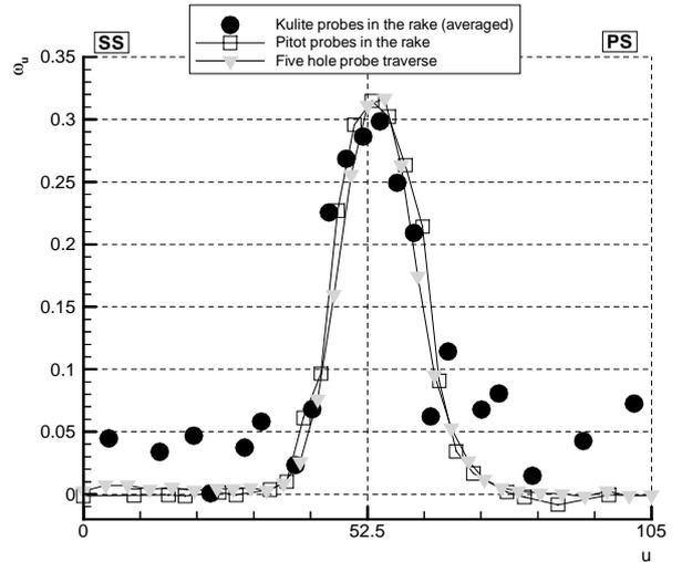
Fig. 7: Total pressure loss coefficient for  $Ma_{2th} = 0.4$ ,  $Re_{2th} = 200,000$ , no turbulence grid
