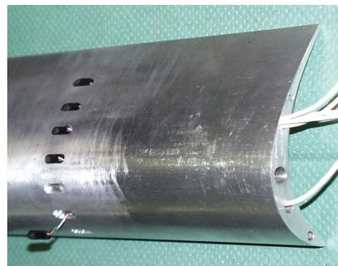
Fig. 2: Blade with LQ-125 Kulite sensors
