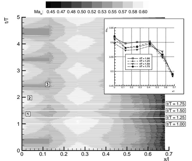
Fig. 9: Space-time diagram of the isentropic Mach number distribution for  $Ma_{2th} = 0.4$ ,  $Re_{2th} = 200,000$ ,  $t_b = 80$  mm,  $U_b = 10.7$  m/s, no grid
