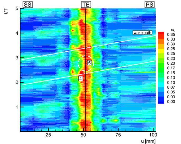
Fig. 12: Space-time diagram of the total pressure loss coefficient for  $Ma_{2th} = 0.4$ ,  $Re_{2th} = 200,000$ ,  $t_b = 80$  mm,  $U_b = 10.7$  m/s, no grid
