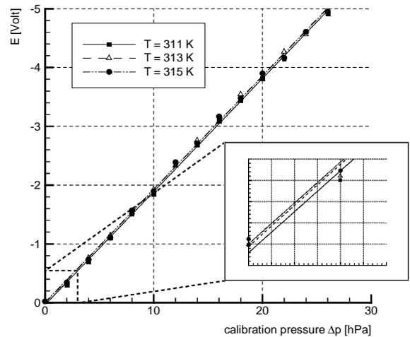
Fig. 4: Calibration data for the *Kulite* sensors in the wake rake
