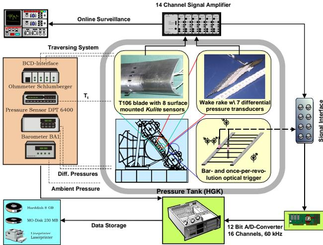
Fig. 5: Schematic drawing of the measurement system
