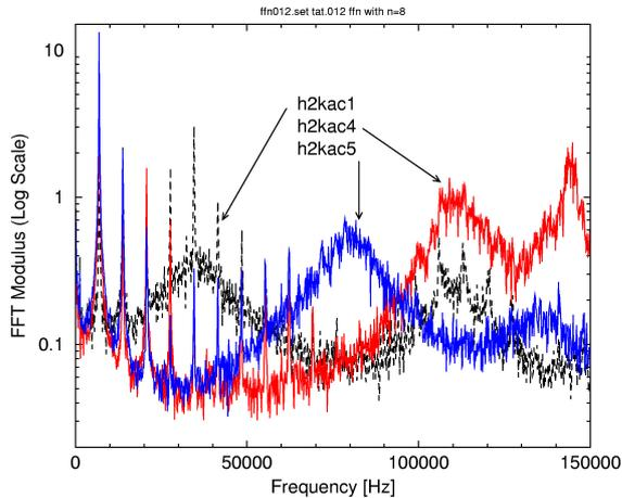
Figure 8: Modulus for FFT of 3 transducers signal when unsteady periodic pressure fluctuations at 4.6 kHz
