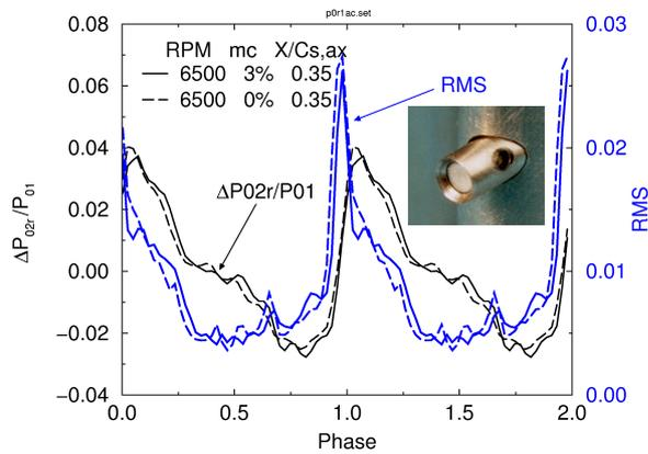
Figure 11: Relative inlet total pressure measured at the rotor leading edge in the turbine test rig.
