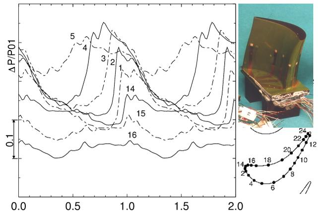
Figure 13: Unsteady static pressure in several points around the rotor blade in a transonic turbine stage.
