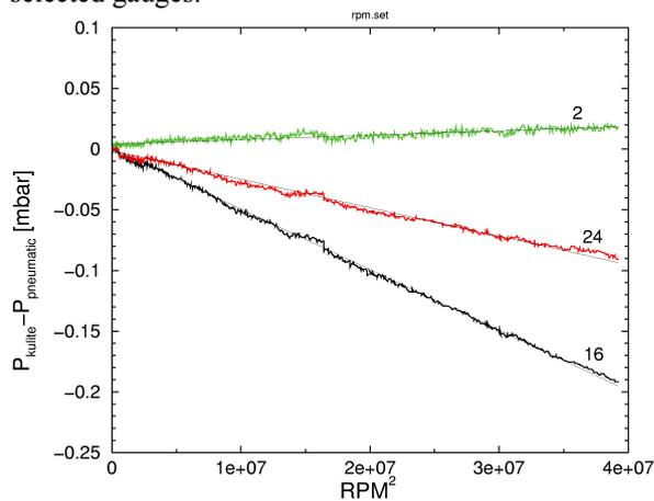
Figure 6: Drifts due to centrifugal force for some sensors
