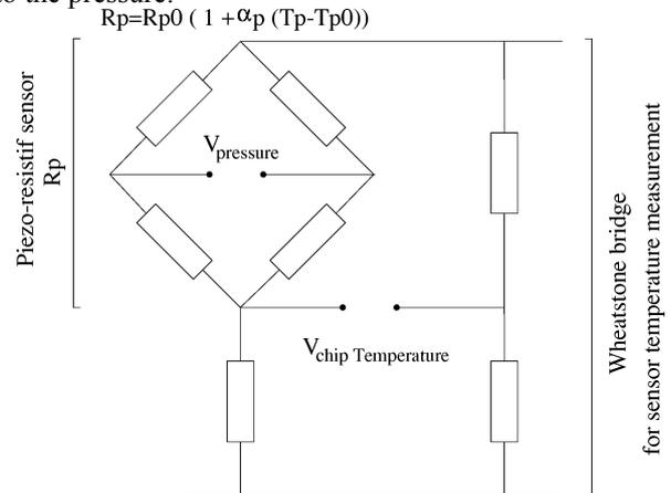
Figure 1: Operating principle of Kulite pressure sensor
