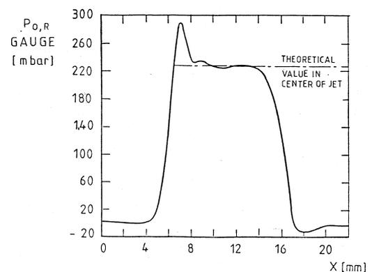
Figure 10: Relative total pressure measured by a Pitot rotating downstream of circular jets.
