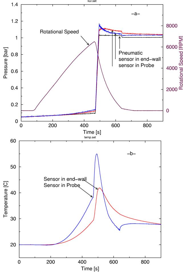
Figure 4: Evolution of: a) the rotational and the pressure (fast response sensor traces are not corrected for temperature) b) the transducer temperature during the transient calibration.
