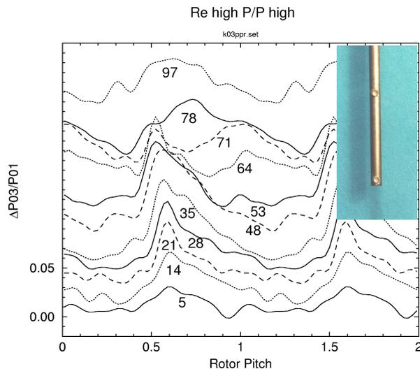
Figure 14: Stage downstream pressure when the rotor operates in the transonic range.
