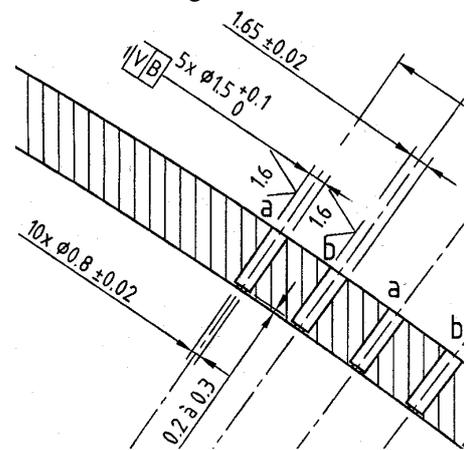
Figure 7: Geometry of the cavity and the orifice dedicated to host the fast response in the tip end-wall.
