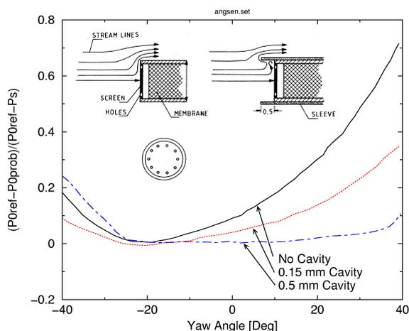
Figure 2: Angular sensitivity of a Pitot probe as a function of the recess of the membrane in the sleeve.
