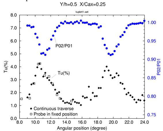
Figure 9: Measuring the turbulence downstream of a vane with a fast response pressure probe.
