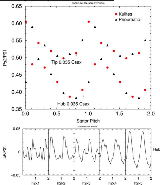
Figure 12: Steady and unsteady static pressure downstream of the vane in a transonic turbine stage.
