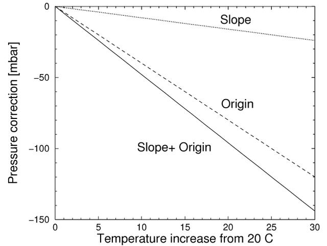
Figure 3: Pressure correction as a function of temperature for an "average" sensor and a voltage output of 1 V (0.830 bar)
