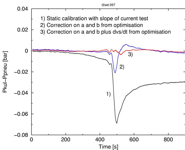
Figure 5: Errors on the sensor in end-wall for the different correction techniques
