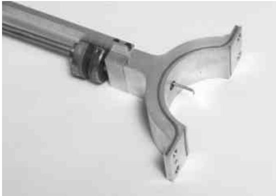
**Fig. 6: Temperature probe at the inset**
