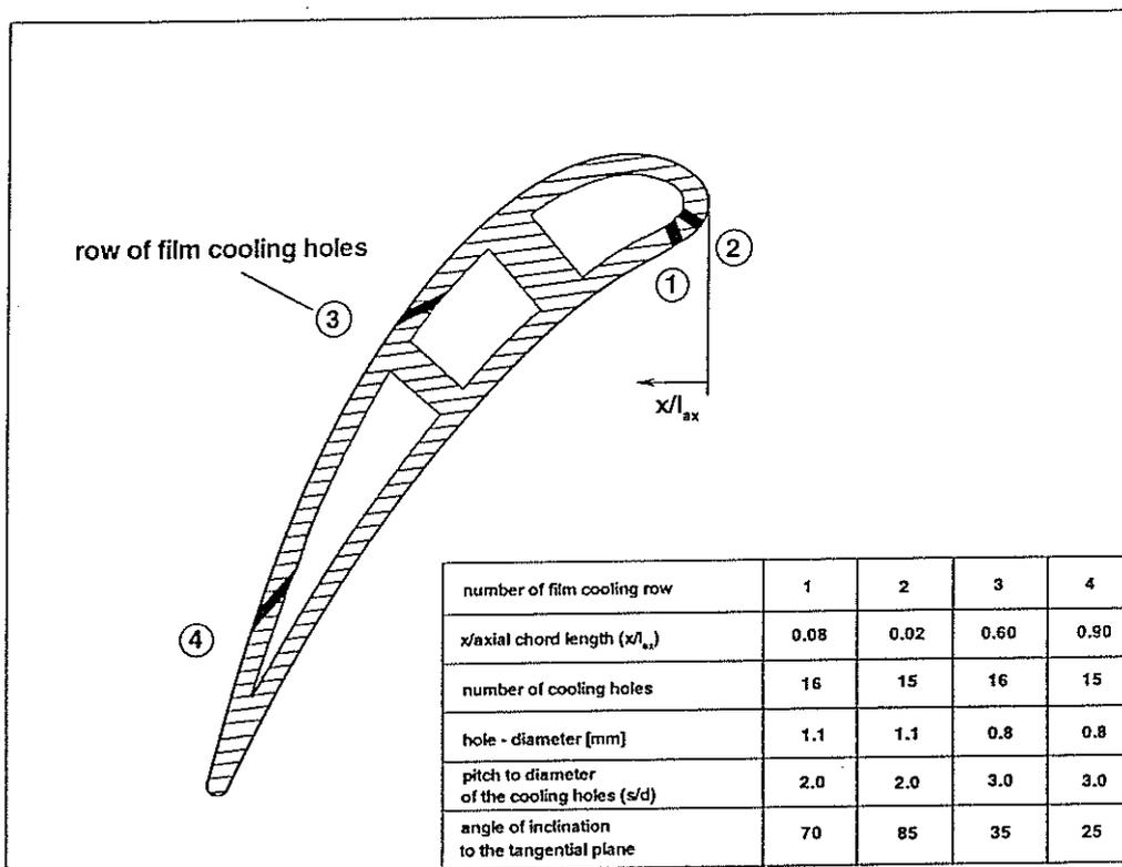
Figure 2: Arrangement of film cooling rows
