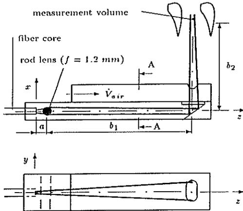
Figure 3: Imaging device with beam path
