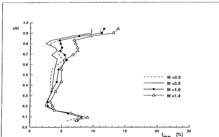
Figure 11: Radial distribution of the kinetic energy loss coefficient  $\zeta_{kin,ex}$
