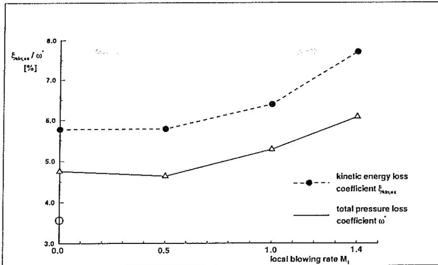
Figure 9: Total pressure loss coefficient  $\omega^*$  and kinetic energy loss coefficient  $\zeta_{kin,ex}$  for different blowing rates
