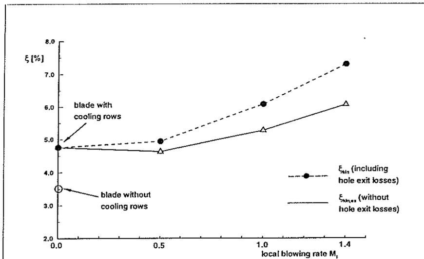
Figure 10: Production of loss of kinetic energy in the blowing holes
