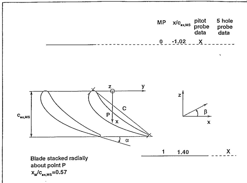
Figure 1: Cascade geometry at mid span and measurement planes
