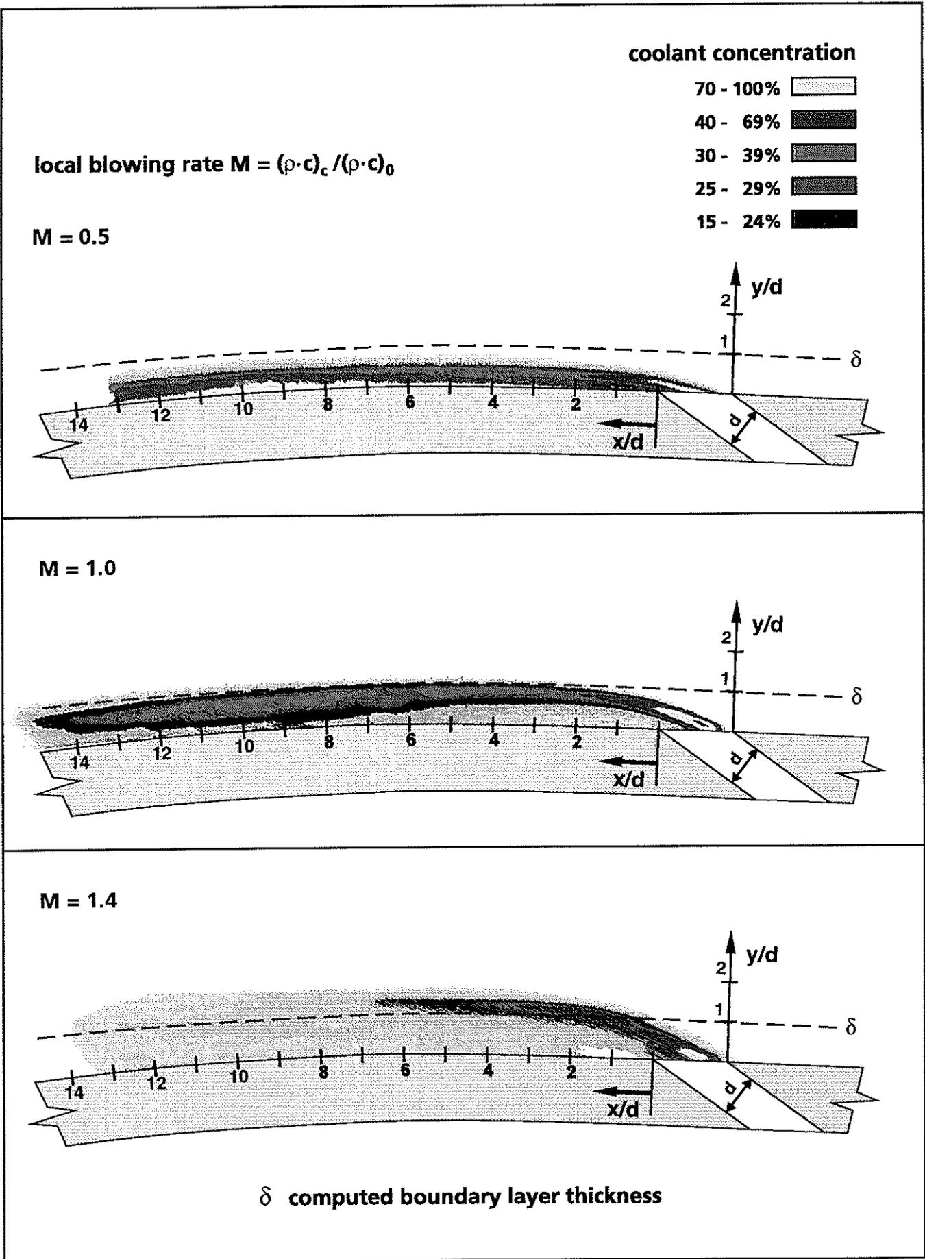
Figure 7: Distribution of cooling air concentration for different blowing rates by pseudo-colored video shots (suction side ejection at row 3,  $x/l = 0.6$ )
