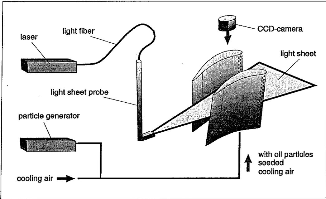
Figure 5: Schematic sketch of visualisation technique
