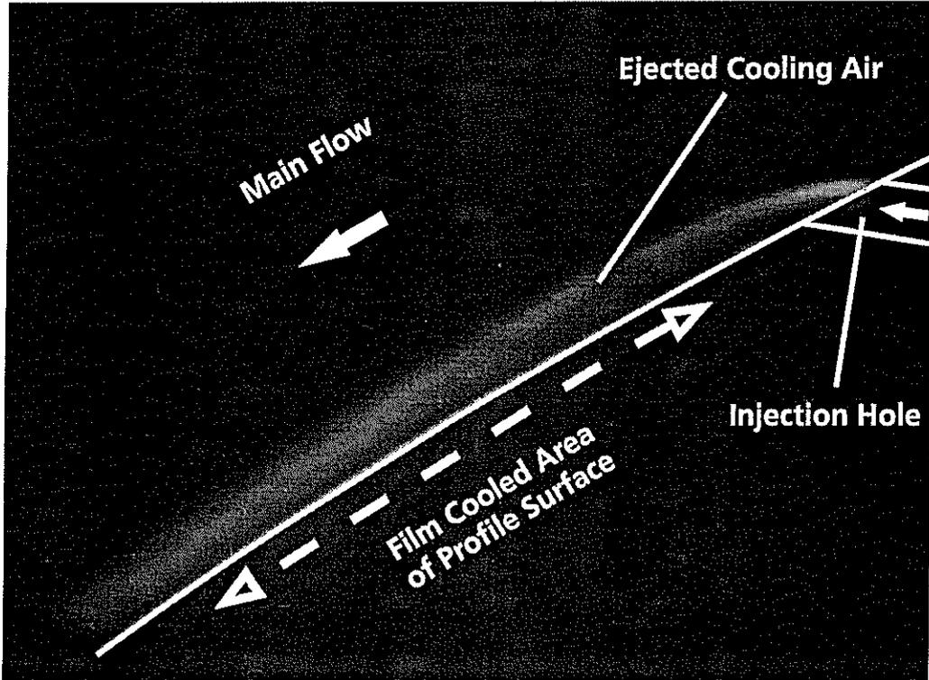
Figure 6: Original video shot of cooling air ejection
