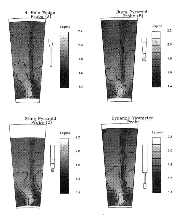
Fig 11: Stagnation pressure ratio measurements taken with the different probes at design speed peak efficiency operation.
