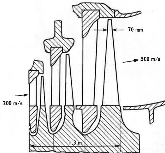
Fig. 5 Wet steam stages of a typical L.P. turbine
