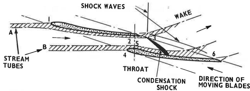
(a) EXAMPLE OF TIP SECTION OF A FINAL STAGE L.P. ROTOR BLADE
