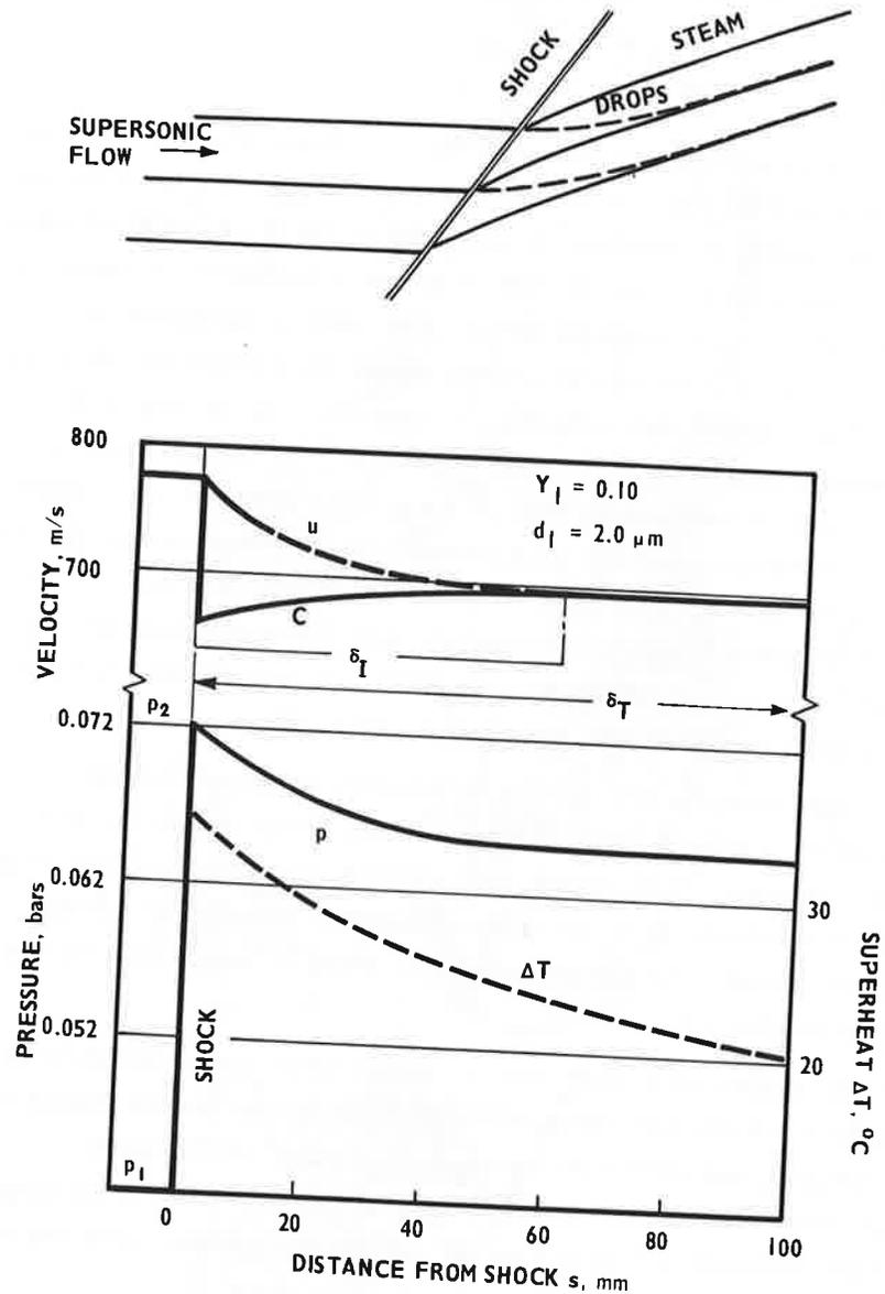
Fig. 3 Wet steam flow through an oblique shock wave
