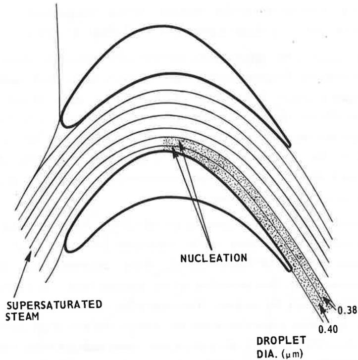
Fig. 2 Two dimensional non-equilibrium flow through an impulse cascade
