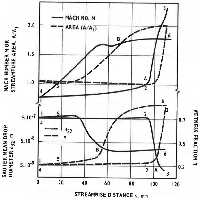
(b) CALCULATED CONDENSATION IN STREAMTUBES
