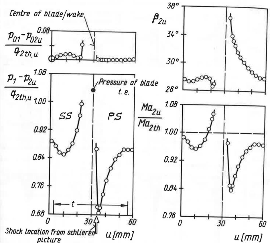
Fig. 4 Local values in the plane of the blade trailing edges,  $e_M/1 = 0$
