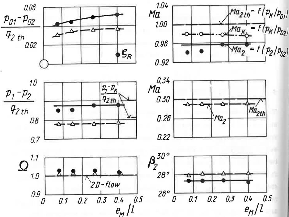
Fig. 6 Average values of flow parameters downstream of the cascade
