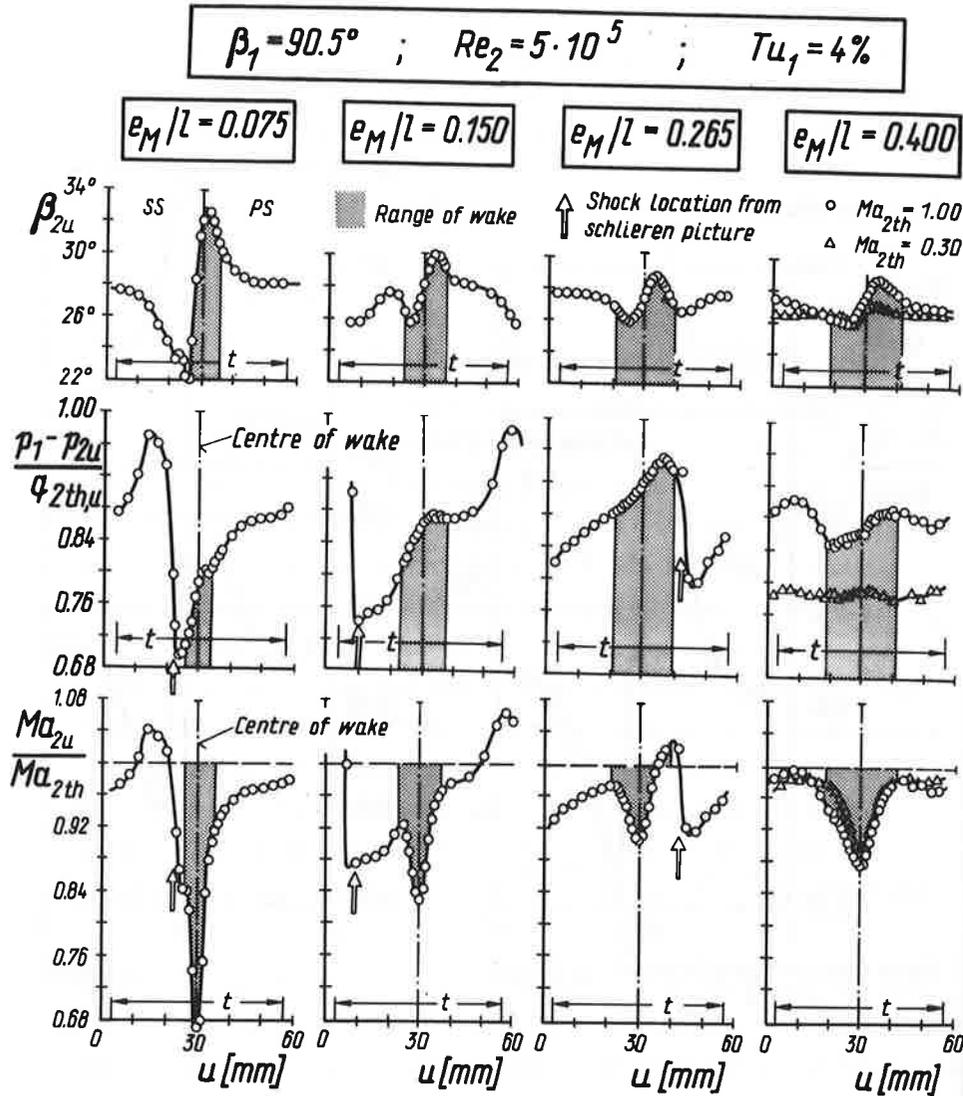
Fig. 5 Local values of flow angle, static pressure change and Mach number downstream of the cascade
