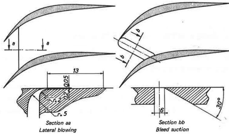
Fig. 6 Control of lateral boundary layers
