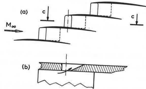
Fig. 9 Supersonic mobile row section. Lateral suction.
