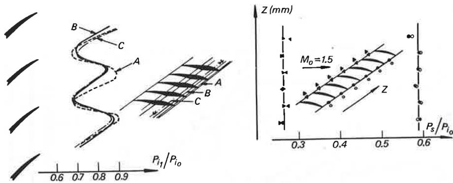
Fig. 4 Supersonic cascade - Test results
