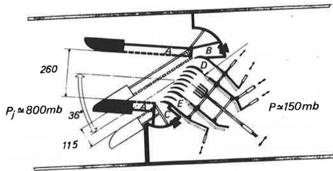
Fig. 1 Test rig for subsonic stator cascade at the S5Ch wind tunnel
