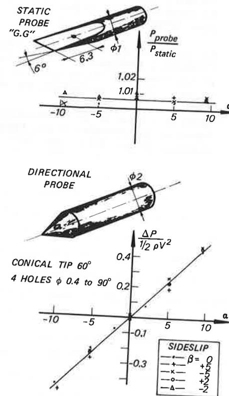
Fig. 11 Static pressure probe and directional probe
