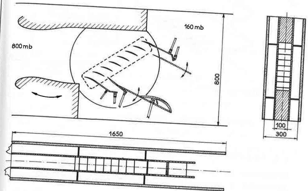
Fig. 3 Test rig for supersonic mobile row section
