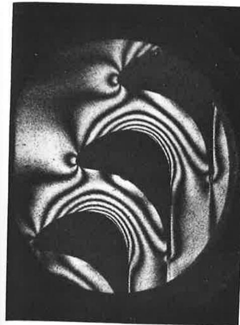
Fig. 9 Lines of constant velocity in a nearly incompressibel flow
