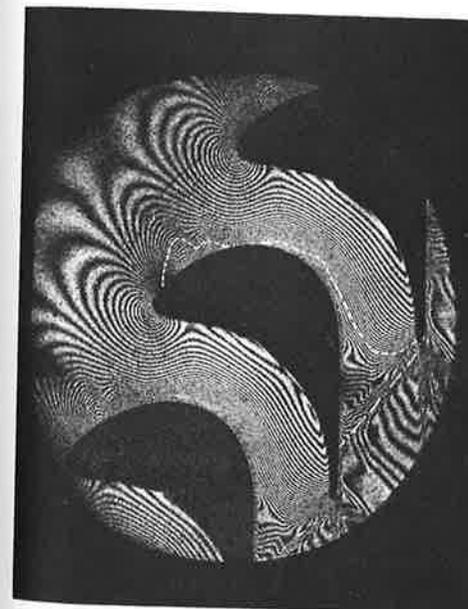
Fig. 10 Lines of constant velocity in a transonic flow
