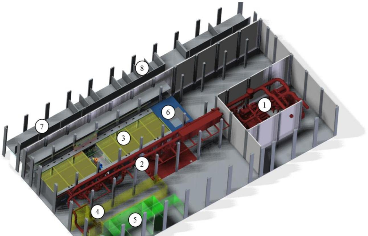
Figure 5: General layout of the new research building; (1) compressor station; (2) primary piping system between compressor station and test rigs; (3) turbomachinery and power plant test cells; (4) linear and annular cascade wind tunnels, aeroacoustic wind tunnel; (5) gas engines; (6) test rig supply; (7) master control room; (8) staff offices
