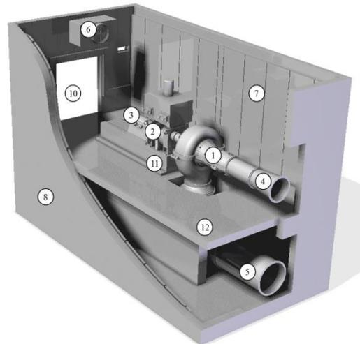
*Figure 6: Layout of the Multi-stage axial turbine test cell; (1) Axial Turbine; (2) el. Generator; emergency brake; (4) inlet section; (5) outlet section; (6) air condition; (7) noise damping elements; (8) reinforced wall; (9) door; (10) vibration-isolated clamping plate*
