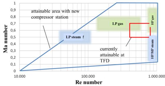
Figure 4: Comparison of Ma number and Re number for typical axial turbines and compressors
