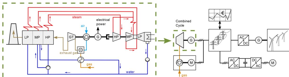
Figure 3: Interrelations between components within the electrical energy supply system by means of a combined cycle power plant
