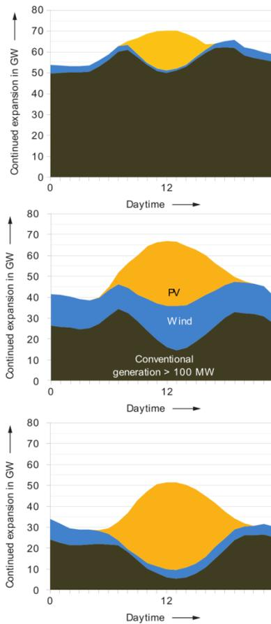
Figure 1: Prognosis for power generation and power supply for the Germany in 2022; top: on Mondays in February, middle: on a Friday in mid may, bottom: on a Saturday at end of May; adapted from Wiese et al. (2013)
